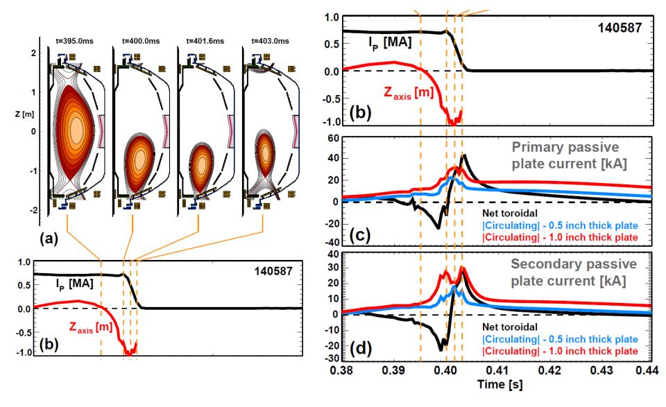
Maximum circulating current of 1" plates is  $\sim$ 1.5x that of 0.5" plate (i.e. < 2x)
