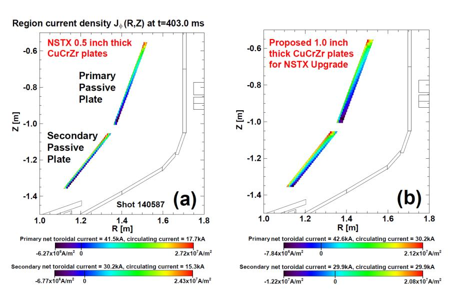
Maximum current density for 1" plates is 75-85% that of 0.5" plate
