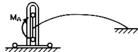
11. Left end restrained against rotation only, right end fixed
