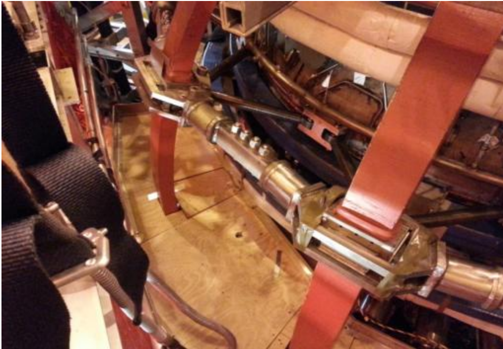
Outer TF Leg turnbuckle supports
