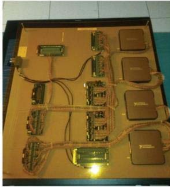
DCPS Autotester Interface Panel Allows local testing of DCPS code
