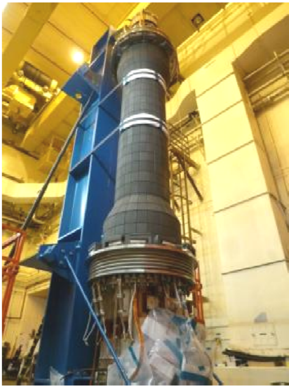
CS Casing being installed over TF/OH bundle
