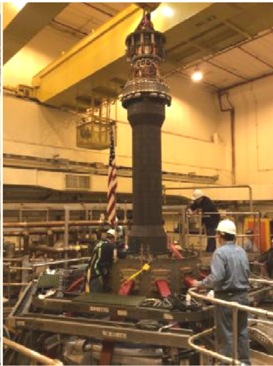
CS assembly being lifted into the machine
