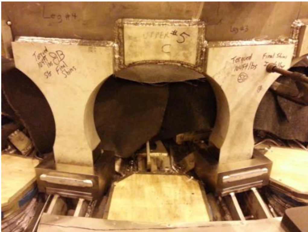
Umbrella legs upgraded from 5/8" to 2" thick
