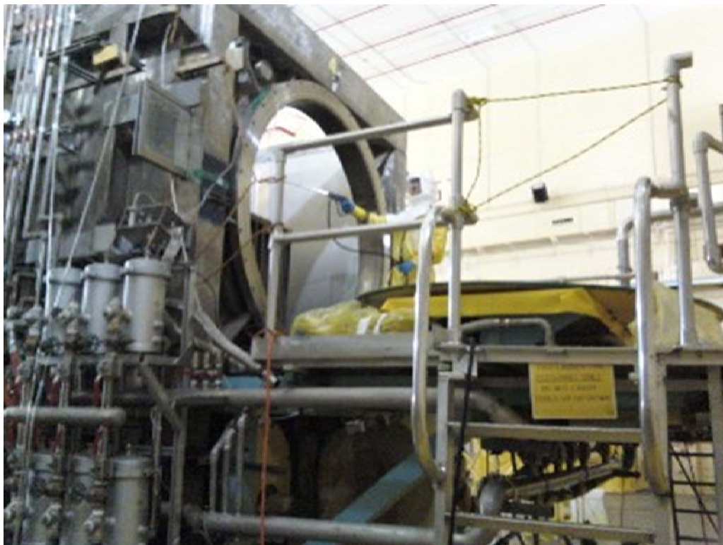
Box decon from lift and from source platform using 25 gallon sprayer and DI water
