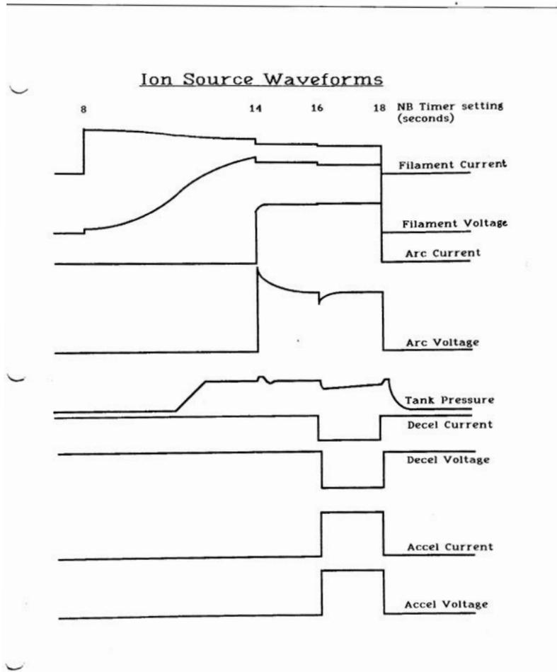
Typical source waveform signatures showing the nesting of filament, gas, arc, decel, and accel for beam formation. Operators monitor and adjust settings manually due to emission limited sources, unregulated filament and arc power supplies, high frequency parasitic oscillations from the HVST, and for adjustments made for experimental requests. Operators assess fault detection, trips, and other anomalies and make corrections between pulses.
