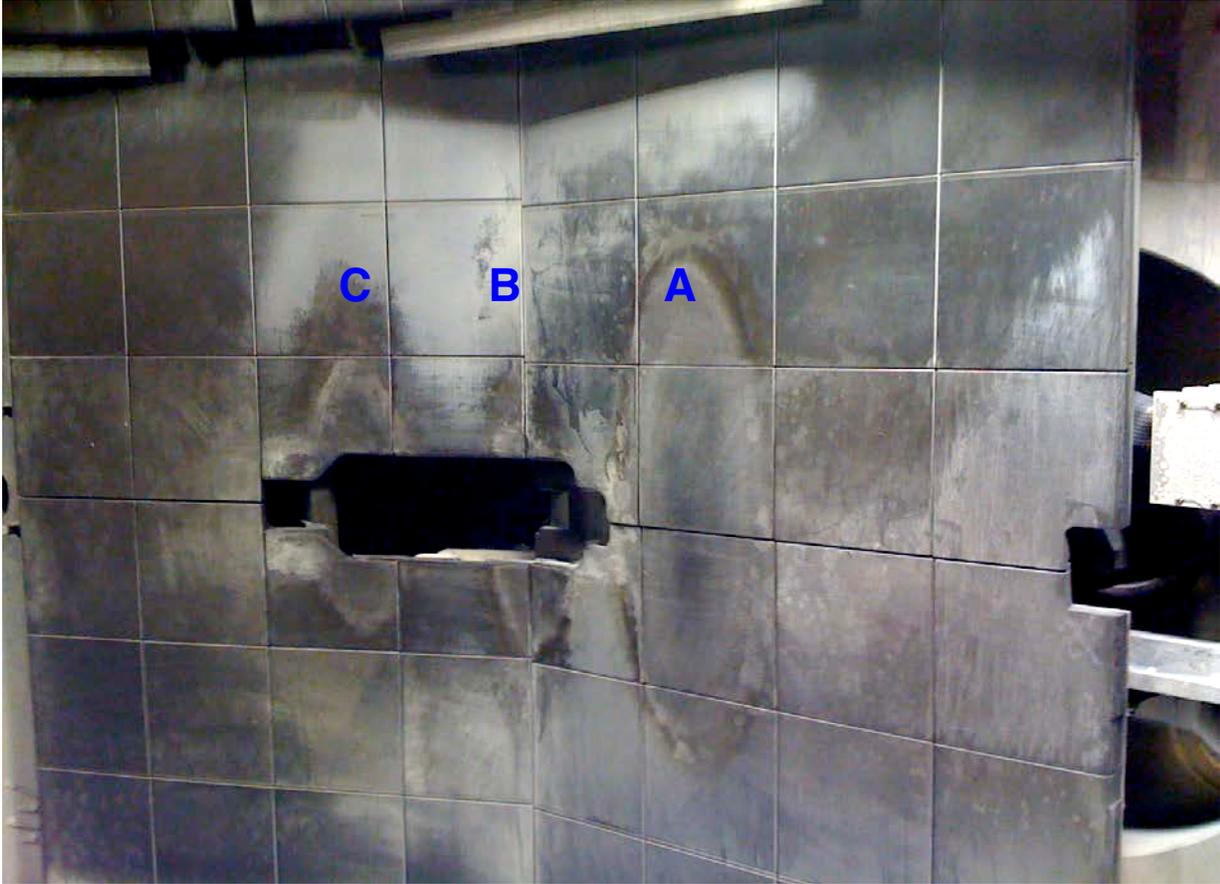
Figure 1: NSTX Armor array showing beam stripping due to neutral beam sources.
