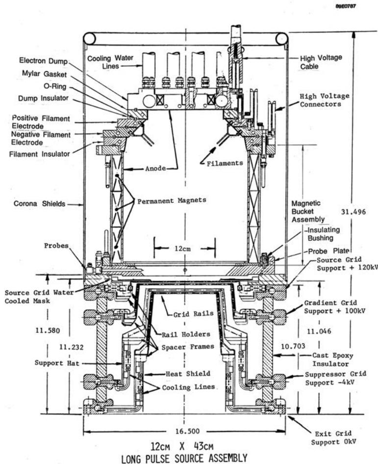
This source has demonstrated its performance on TFTR and TFTR DT from 1987 to 1997 and on ten years operating experience on NSTX from 2000 to the present. The source is rated for 120 keV, 70 Amps, 2 seconds, with a duty factor of .017. The full energy, half energy, and third energy components arise from the reduction of D<sub>2</sub> covalent bonds to ions in the arc plasma.
