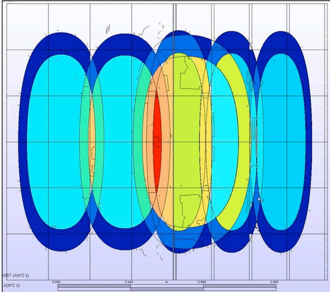
Figure 2: Overlapping beam profiles, showing placement and heat flux.
