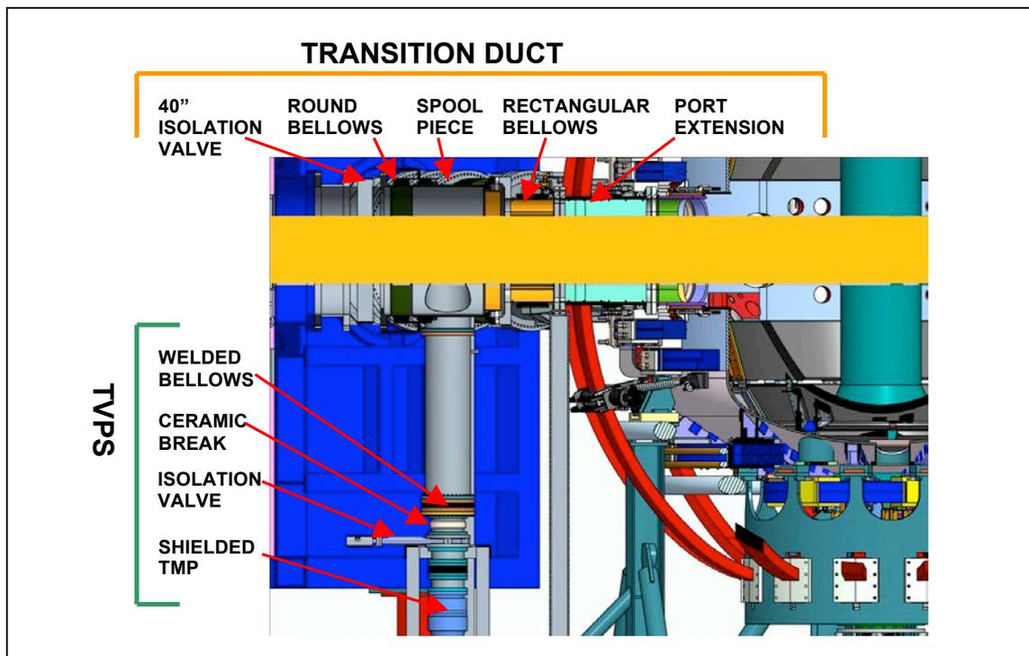
Figure 2: NB2 Transition duct and TVPS pumps below
