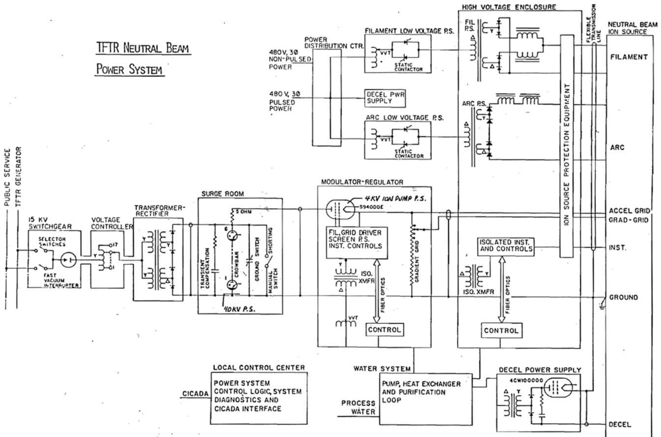
The HVEs will be moved from Test Cell Basement. New triax cables will be installed from M/R to HVE in the NTC. The single point grounding system used for BL1 will be employed on BL2 also. The large elephant trunk transmission lines have been salvaged from TFTR and will be reused to connect the HVE to the source platform pressure plate connector. The power cabling is otherwise conventional conductors and sizes.
