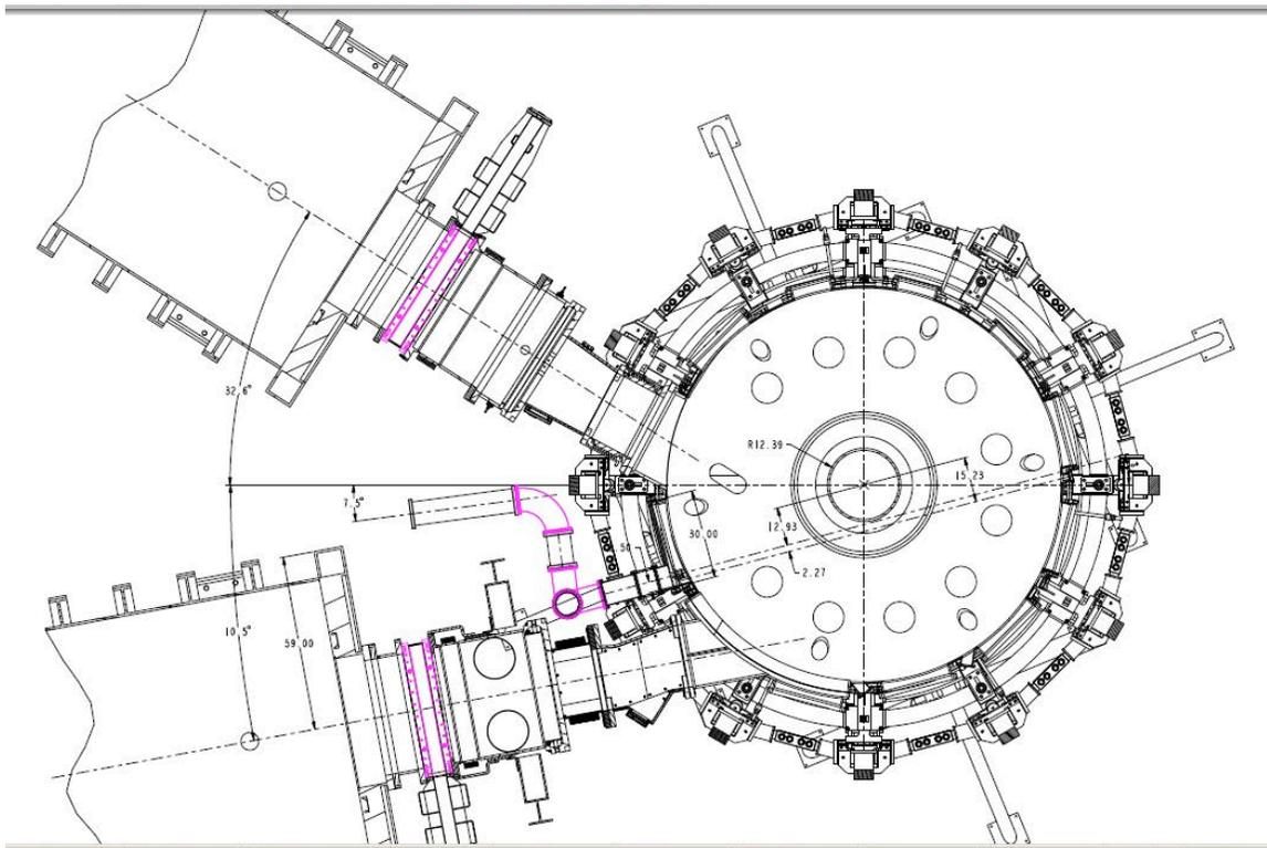
MPTS View across machine with new Center Stack diameter and enlarged Bay L port
