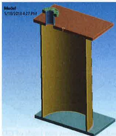
Fig. 6-1 The cross-section view of GDS expansion tank The cross-section view of GDS expansion tank is shown in Figure 6-1.
