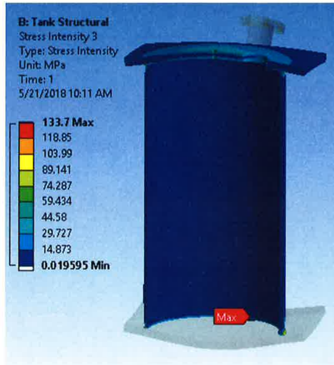
Fig. 7-1 The stress intensity of GDS expansion tank
