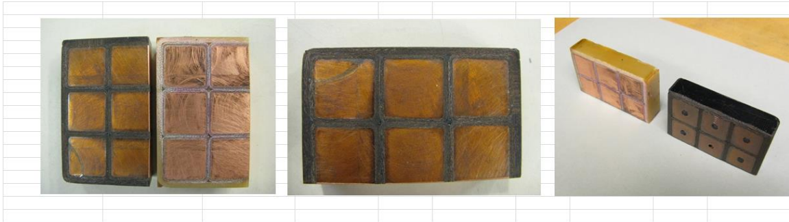
Figure 10.1-Samples “Cooked “ for 24 Hr. , Peak Temp=225C
