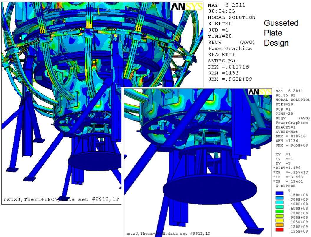
Figure 9.2-2 Scenario 13 Gusseted Plate Pedestal Stresses
