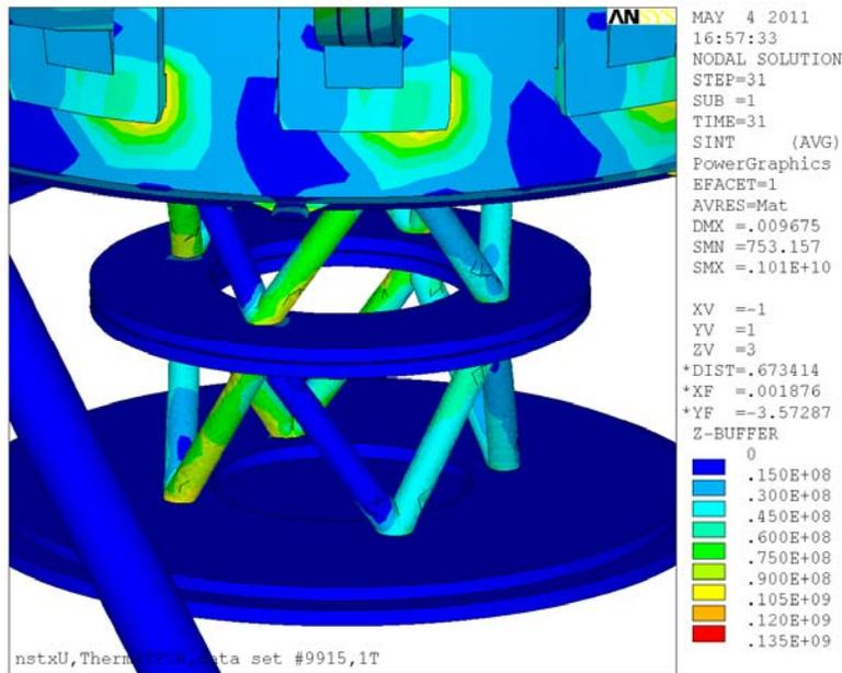
Figure 9.2-4 Scenario 15 "Vee" Pipe Pedestal Stresses
