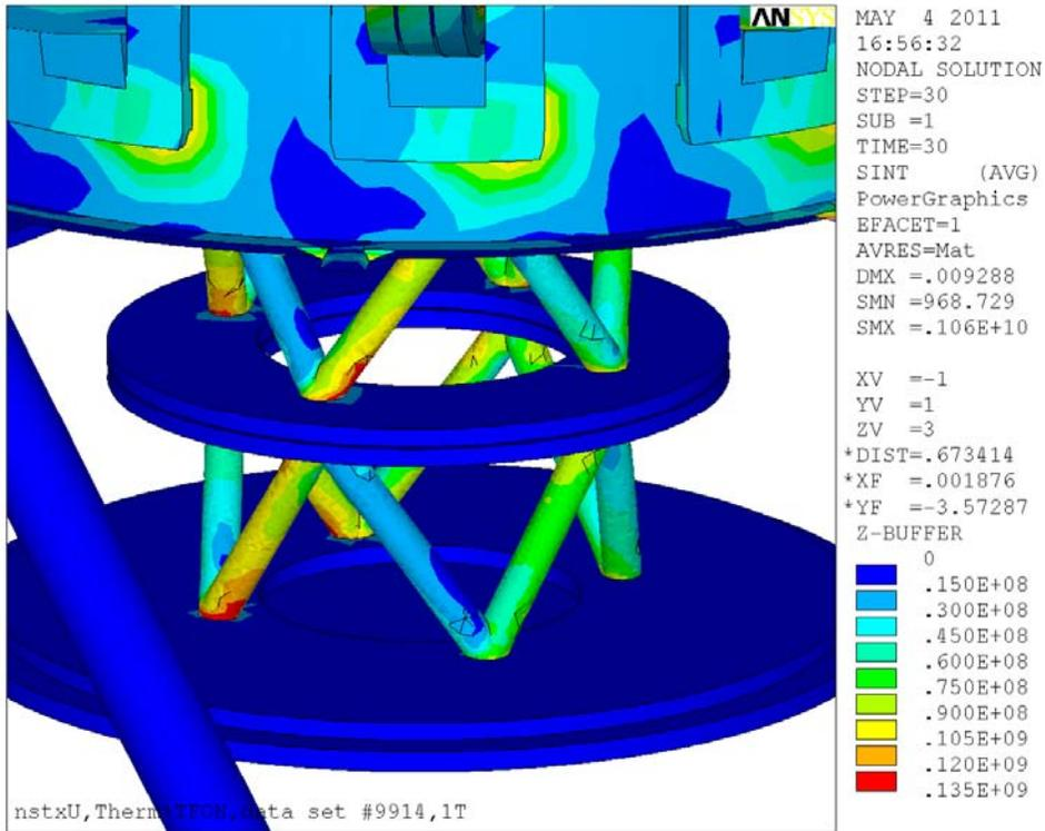
Figure 9.2-3 Scenario 14 "Vee" Pipe Pedestal Stresses
