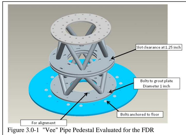
Figure 3.0-1 "Vee" Pipe Pedestal Evaluated for the FDR
