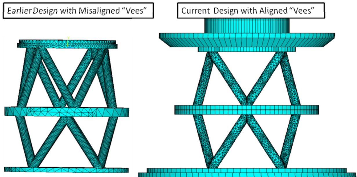
Figure 6.0-2 "Vee" Pipe models -Misaligned and Aligned
