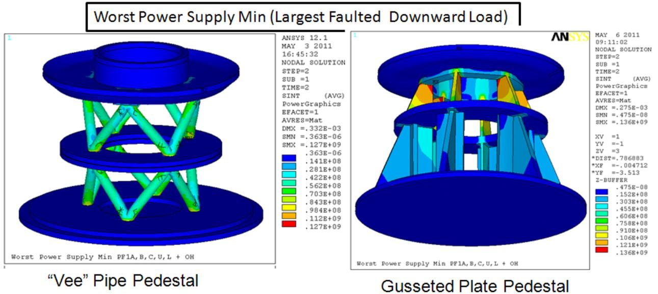
Downward and Normal and Faulted Stresses are acceptable for both pedestal concepts. Stresses are almost the same for both concepts.
