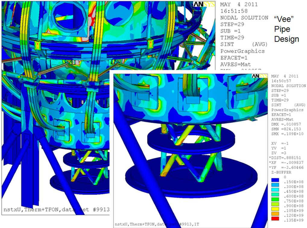
Figure 9.2-1 Scenario 13 "Vee" pipe Pedestal Stresses
