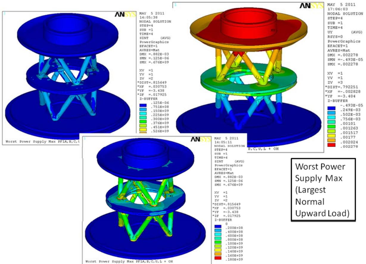
Upward Normal and Faulted Stresses are acceptable for both pedestal concepts. Stresses are similar for both concepts.
