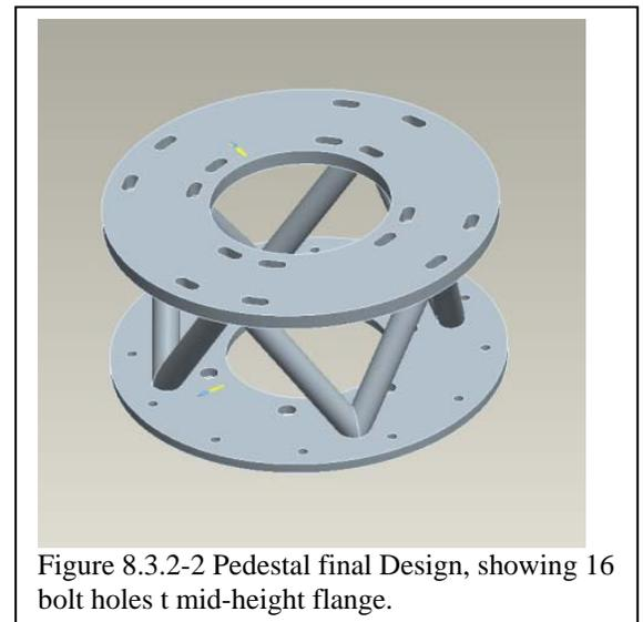
Figure 8.3.2-2 Pedestal final Design, showing 16 bolt holes t mid-height flange.
