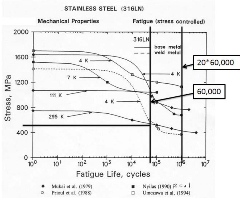
Figure 7.0-3 Fatigue S-N Curve for 316 Stainless Steel
