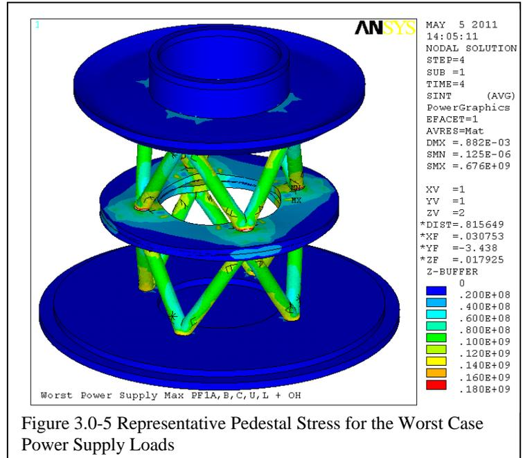
Figure 3.0-5 Representative Pedestal Stress for the Worst Case Power Supply Loads
