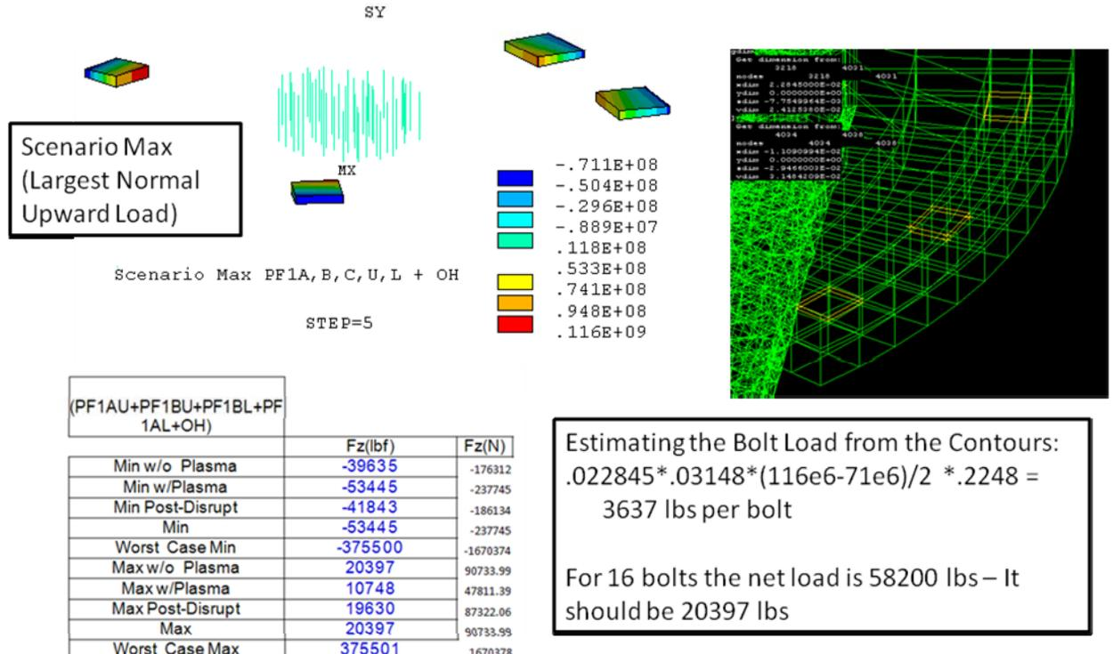
Figure 8.3.2-3 Bolt Loads including the non-linear prying/bending action on the Bolts - -
