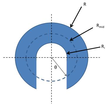
The maximum radius for contact is R (0.125") and the cut-out feature corresponds to features in the lock-bar with a  $R_i=0.083$ ". One estimate for the contact line may be at the mid-point between  $R_i$  and R which corresponds to  $R_{mid}=0.104$ ". The half-angle of the cut is given as:
