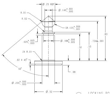
The pin head geometry has not changed since the prototype process:
