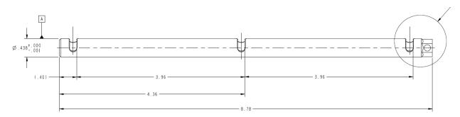
A simple stress estimate is made assuming a bar in bending with a symmetry point half-way between lock pins. The moment applied is 3.96/2" with the full load of 189 lbf resulting in 373.9 lbf-in.
