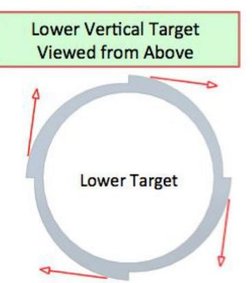
This image is from NSTX-U-RQMT-SRD-003-02 giving the sense of the fish-scale steps. Moving clockwise, there is a step outward in major radius. This sense matches the current drawing.
