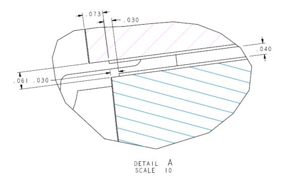
This image is taken from E-ED1459 at zone I-8 showing a section view from above looking downward at the HTP. Moving clockwise, there is a step outward in major radius.
