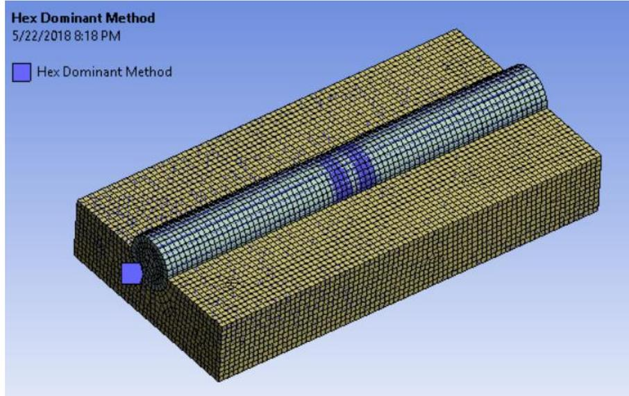
Figure 7.0-11. Workbench model of rod and graphite block
