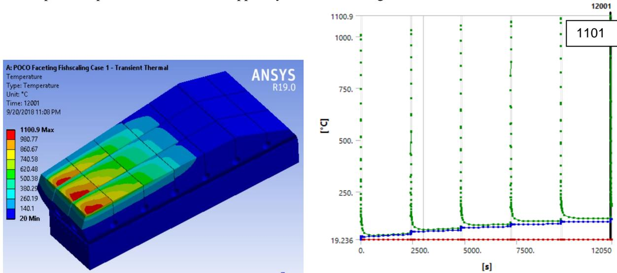
Figure 9.0-2 The temperature ratcheting and peak temperature at 12001s with OBD12 POCO Case 1
