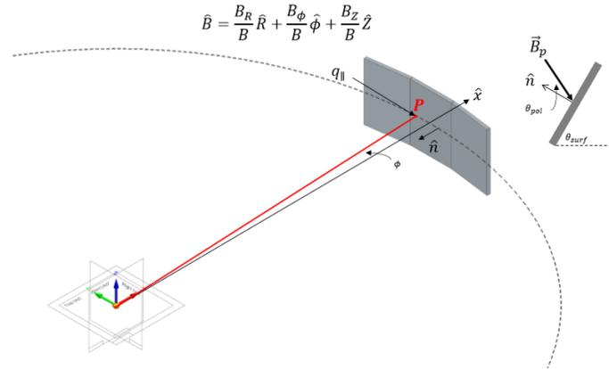
Figure 7.0-1 The scheme for a vertical plate, faceted divertor (from Reinke [6])
