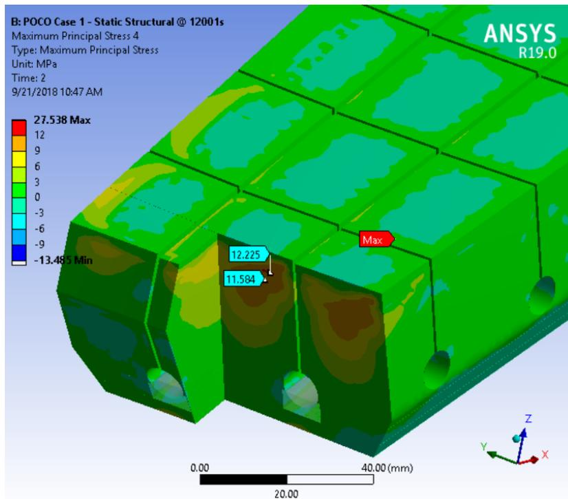
Figure 9.0-5 The max principal stress of tile at 12001s with OBD12 POCO Case 1
