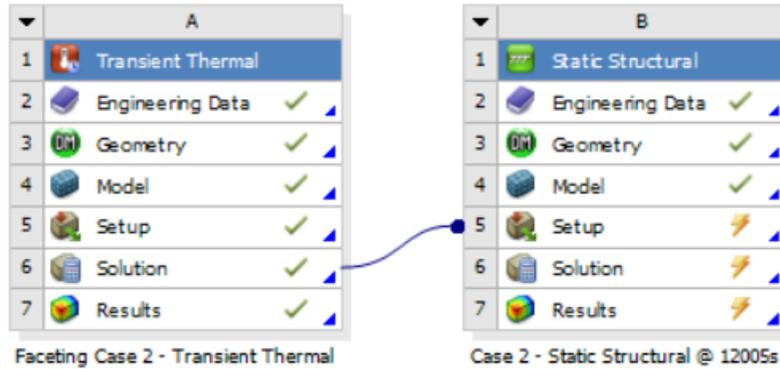
Figure 7.0-9 The combined structural model with the imported thermal loads
