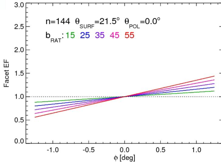
Figure 7.0-2 Faceting Enhancement Factors for OBD12 with angles of incidence from Reinke
