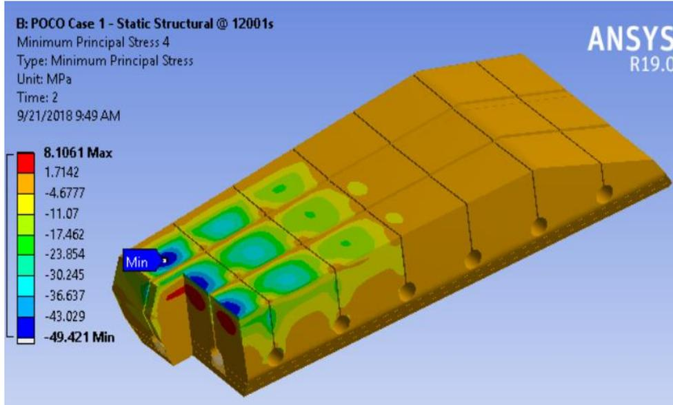
Figure 9.0-4 The minimum principal stress of tile at 12001s with OBD12 POCO Case 1
