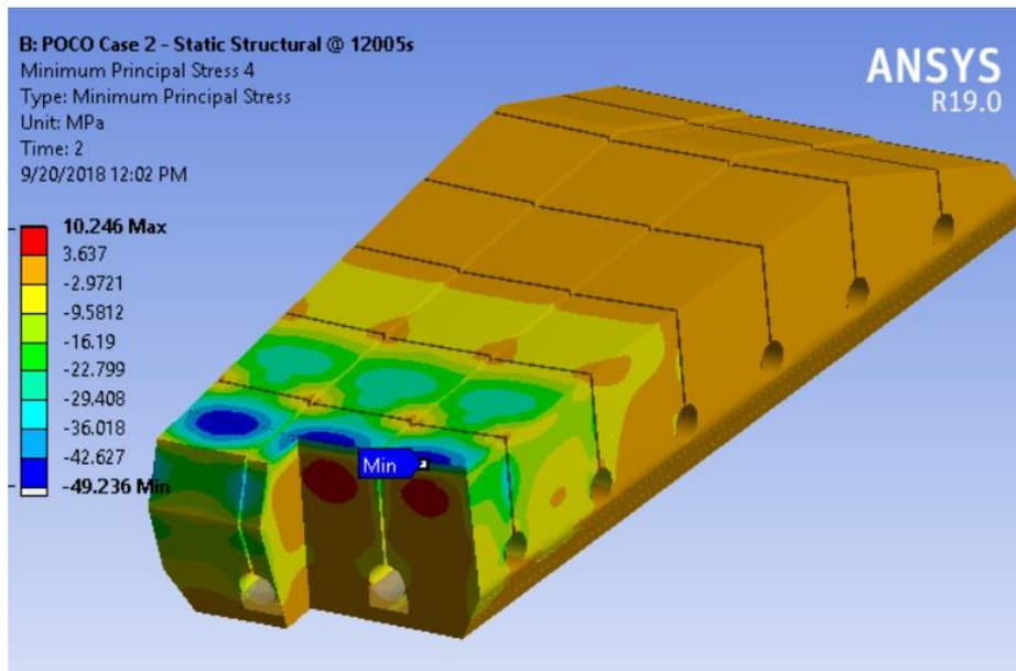
Figure 9.0-8 The minimum principal stress of tile at 12005s with OBD12 POCO Case 2
