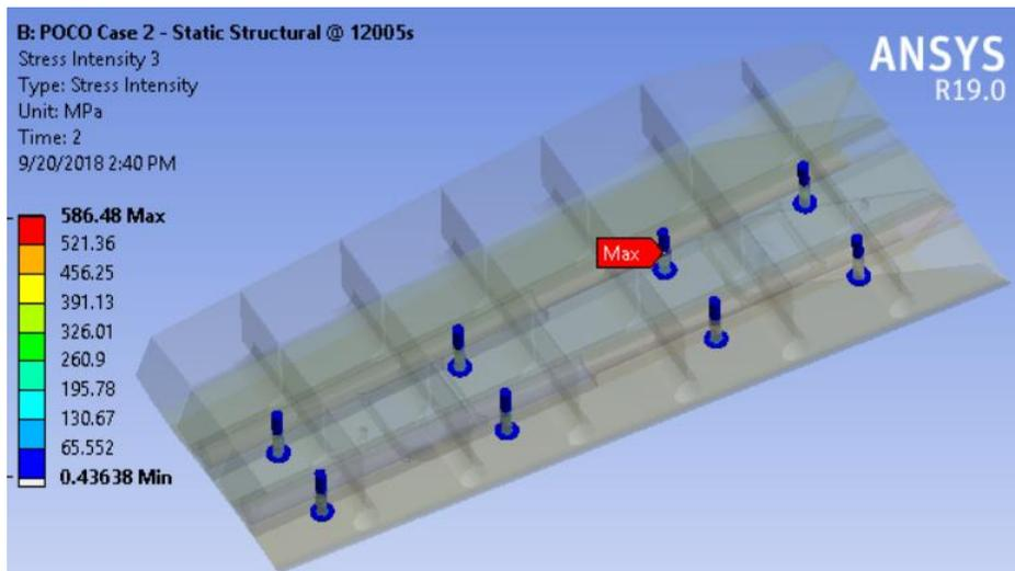
Figure 9.0-11 The stress of bolts at 12005s with OBD12 POCO Case 2
