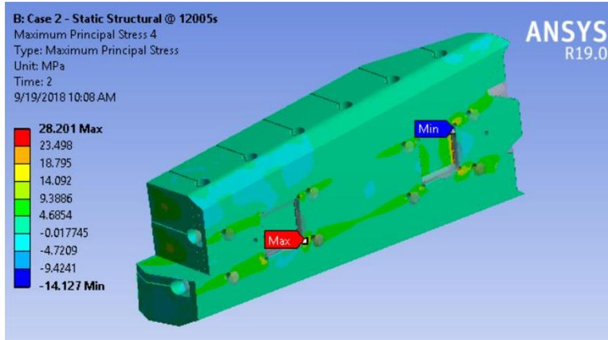
Figure 8.0-10 The max principal stress of tile at 12005s with OBD12 **Sigrafine** Case 2
