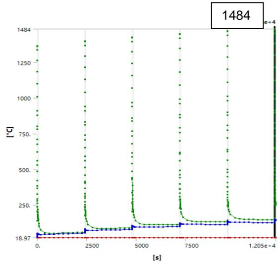
Figure 8.0-1 The temperature ratcheting and peak temperature at 12001.5s with OBD12 Case 1
