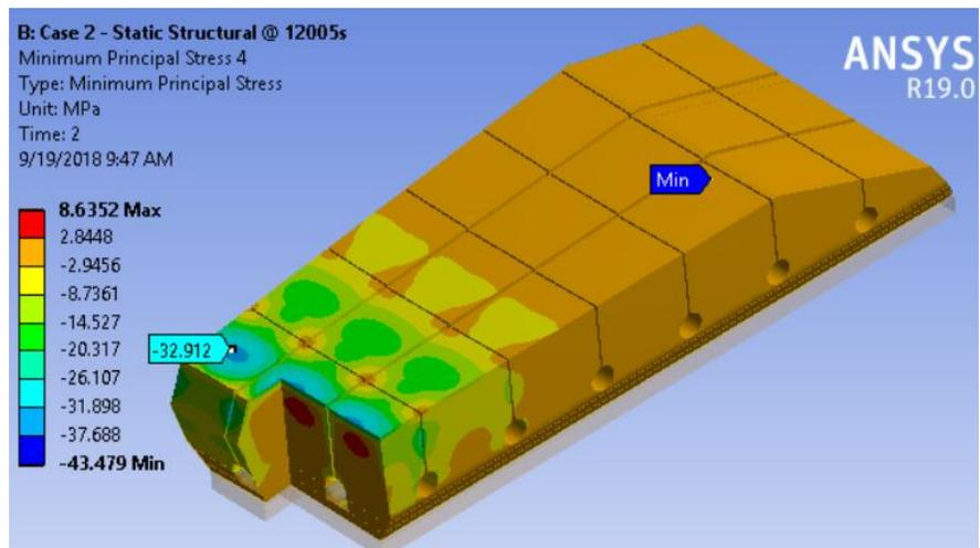
Figure 8.0-9 The minimum principal stress of tile at 12005s with OBD12 **Sigrafine** Case 2
