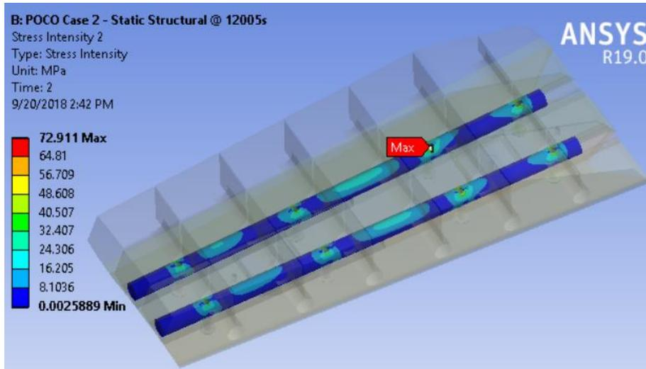
Figure 9.0-10 The stress of rods at 12005s with OBD12 POCO Case 2
