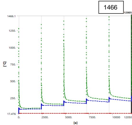
Figure 8.0-3 The temperature ratcheting and peak temperature at 12005s with OBD12 Case 3
