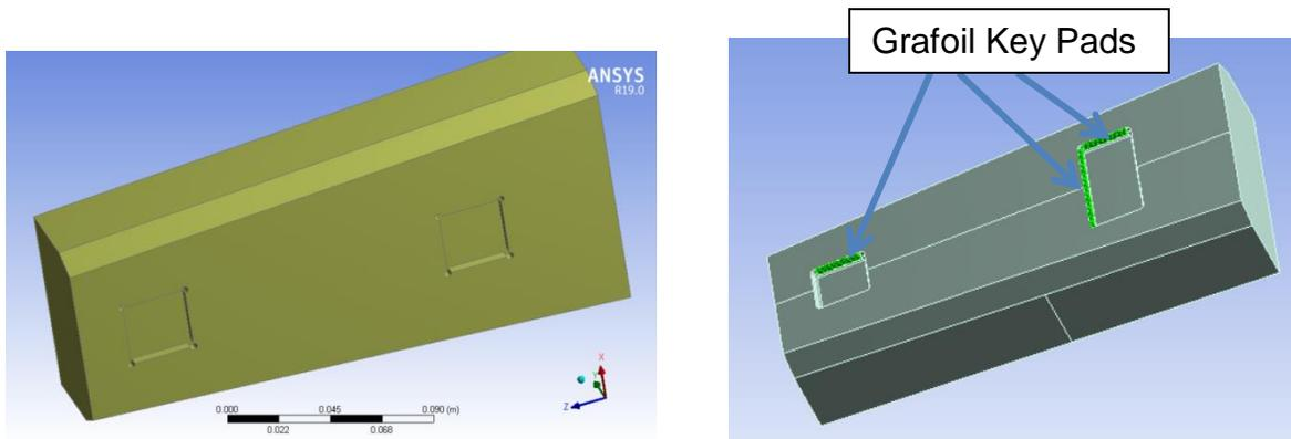
Figure 7.0-14. Original vs new simplified key model (halo restraints)
