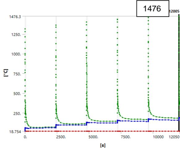
Figure 8.0-4 The temperature ratcheting and peak temperature at 12005s with modified faceting OBD12 Case 2.
