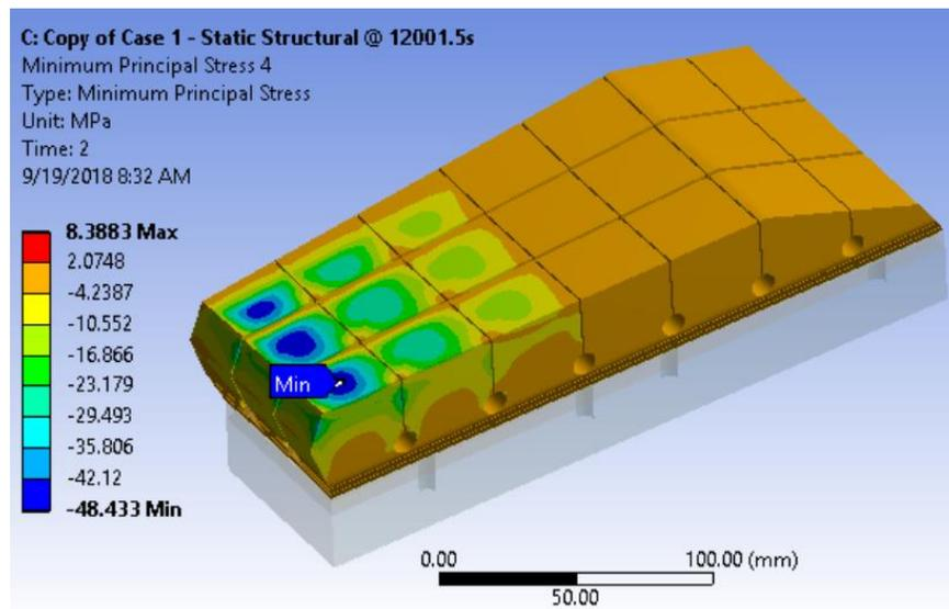
Figure 8.0-5 The minimum principal stress of tile at 12001.5s with OBD12 **Sigrafine** Case 1
