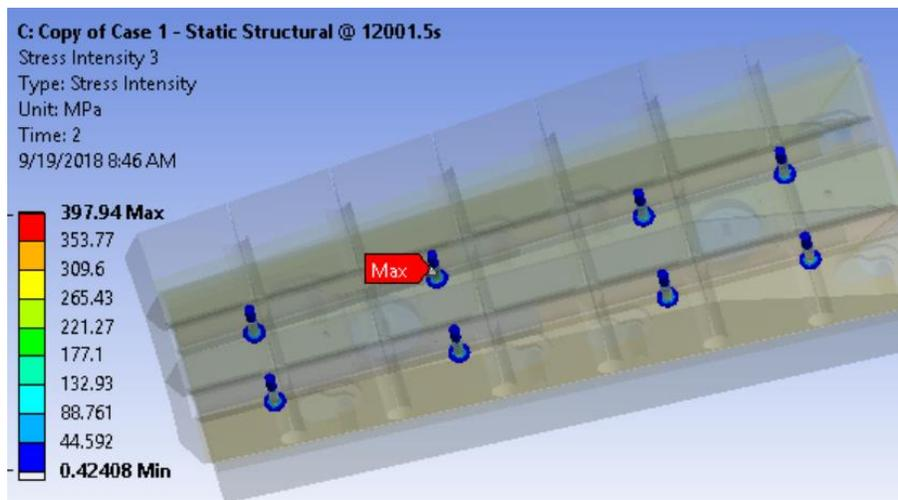
Figure 8.0-8 The stress of bolts at 12001.5s with OBD12 **Sigrafine** Case 1
