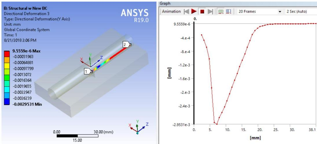
Figure 7.0-13. Vertical Displacement of tile along the contact path.
