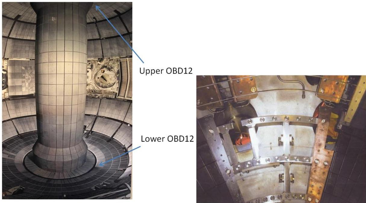
Figure 5.0-1 The original OBD Row 1&2 Tiles and underneath mounting BBQ rails without cooling.
