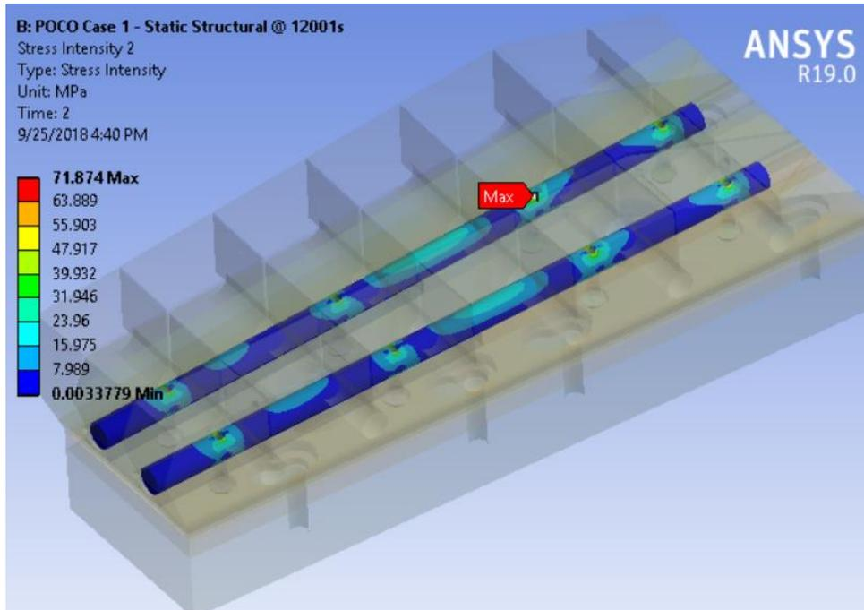
Figure 9.0-6 The stress of rods at 12001s with OBD12 POCO Case 1
