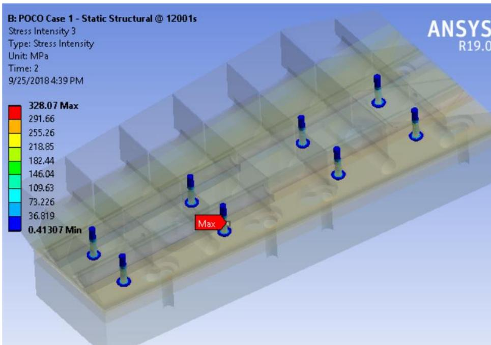
Figure 9.0-7 The stress of bolts at 12001s with OBD12 POCO Case 1
