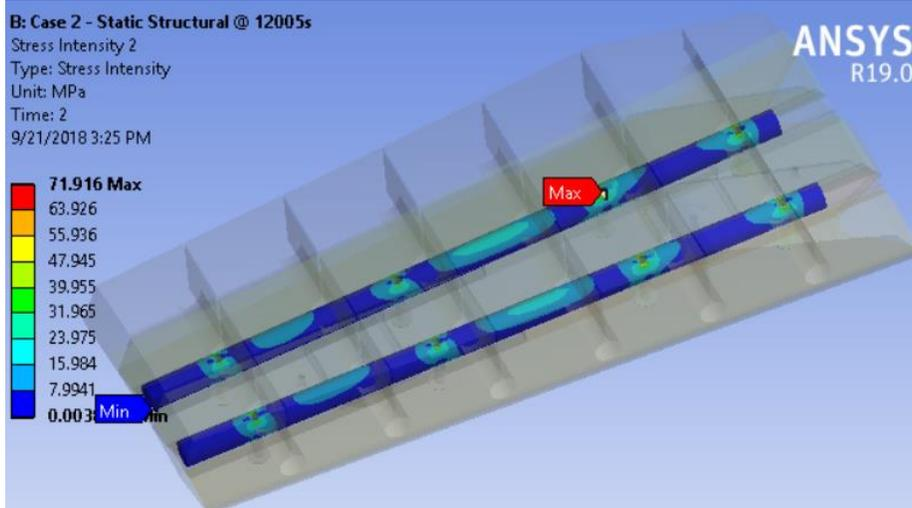
Figure 8.0-11 The stress of rods at 12005s with OBD12 **Sigrafine** Case 2
