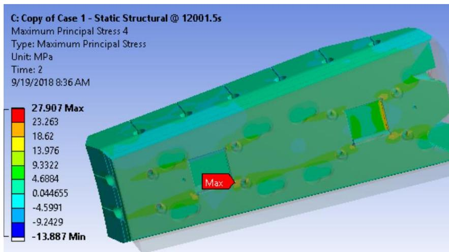
Figure 8.0-6 The max principal stress of tile at 12001.5s with OBD12 **Sigrafine** Case 1
