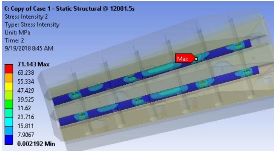
Figure 8.0-7 The stress of rods at 12001.5s with OBD12 **Sigrafine** Case 1
