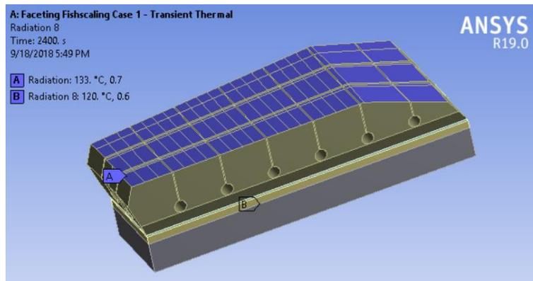
Figure 7.0-8 The radiation settings of the thermal model for OBD12
