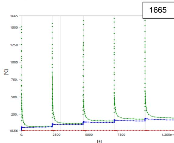
Figure 8.0-2 The temperature ratcheting and peak temperature at 12005s with OBD12 Case 2
