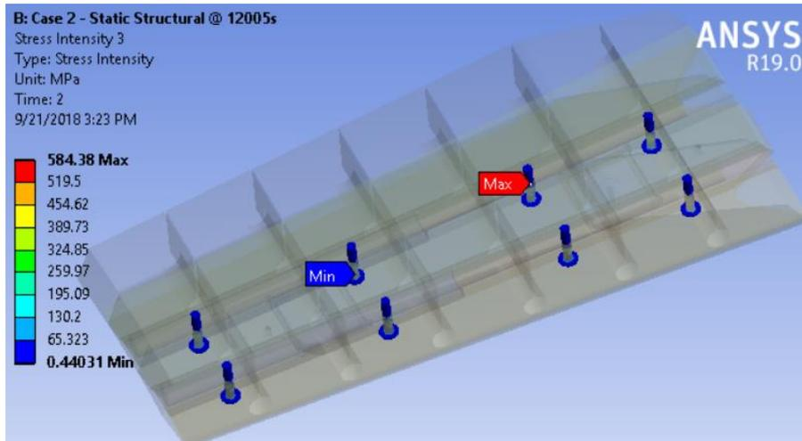
Figure 8.0-12 The stress of bolts at 12005s with OBD12 **Sigrafine** Case 2
