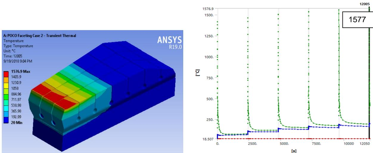
Figure 9.0-3 The temperature ratcheting and peak temperature at 12005s with OBD12 POCO Case 2
