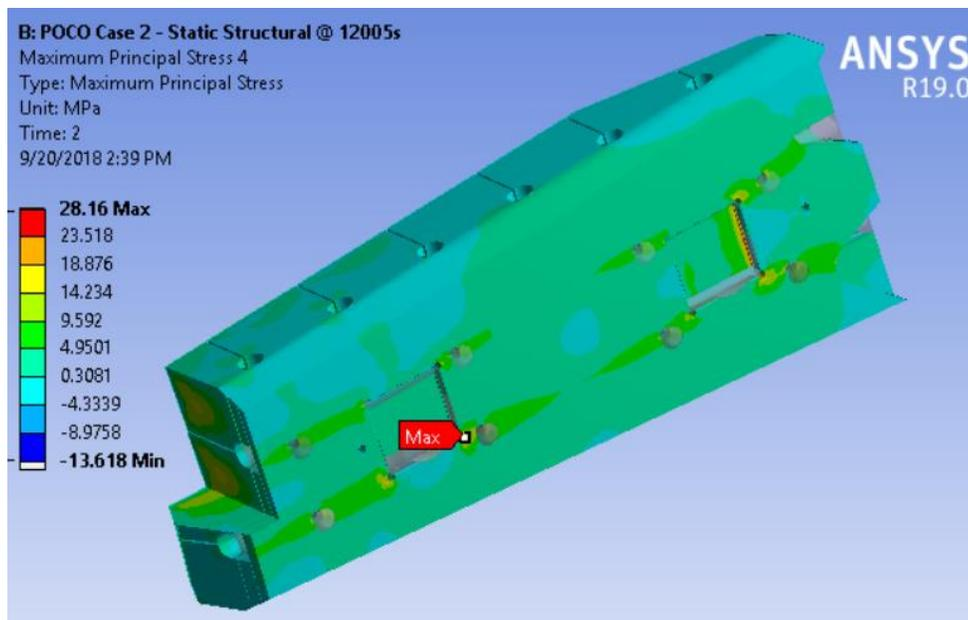
Figure 9.0-9 The max principal stress of tile at 12005s with OBD12 POCO Case 2
