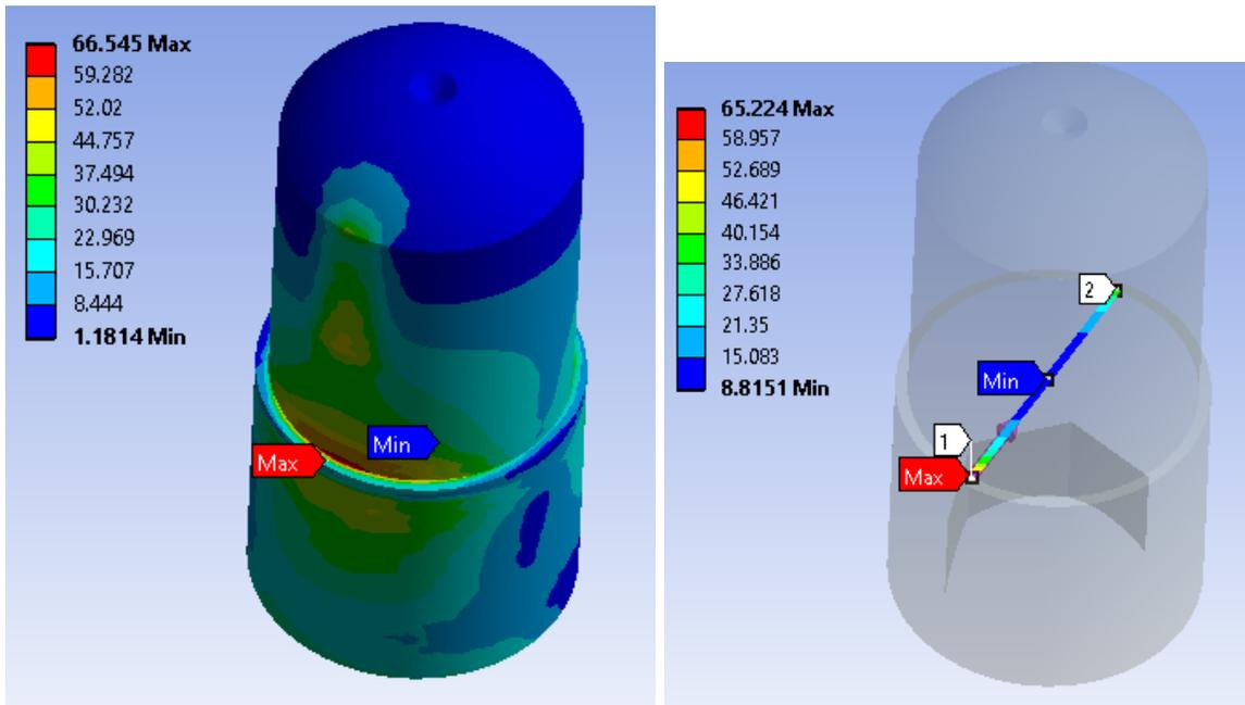
Figure 22: Variant Tile Shear Pin Stresses
