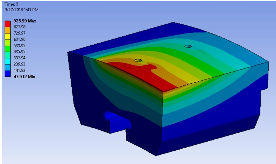
Figure 8: Default Tile Thermal Results at End of 5 Seconds Flux Shot
