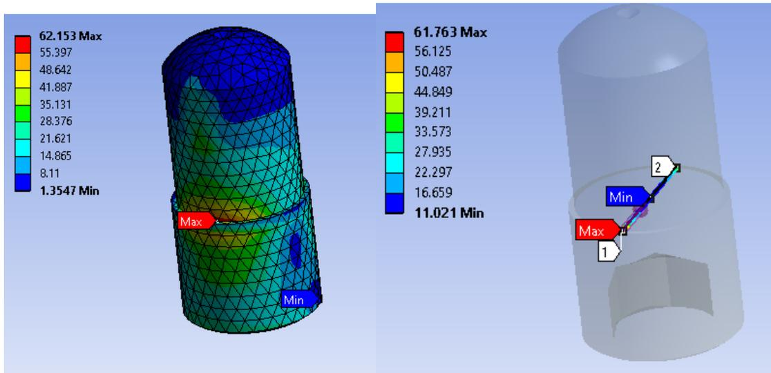
Figure 17: Default Tile Shear Pin Stresses
