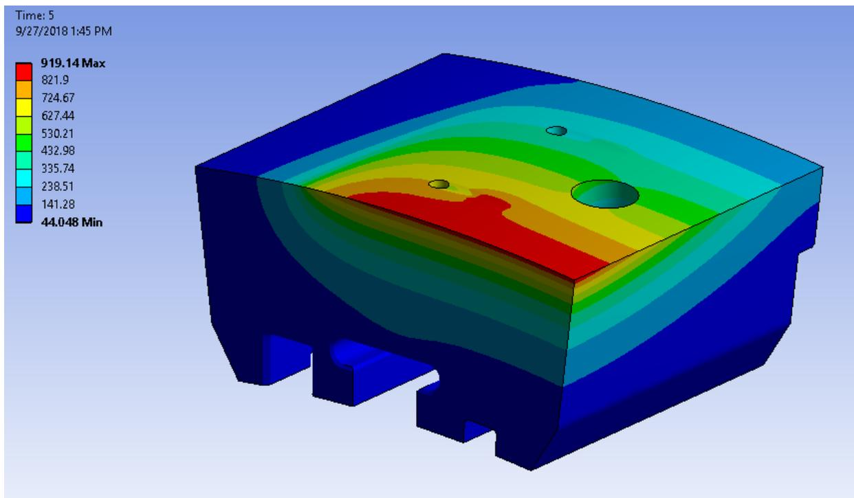
Figure 11: Variant Tile Thermal Results at End of 5 Seconds Flux Shot
