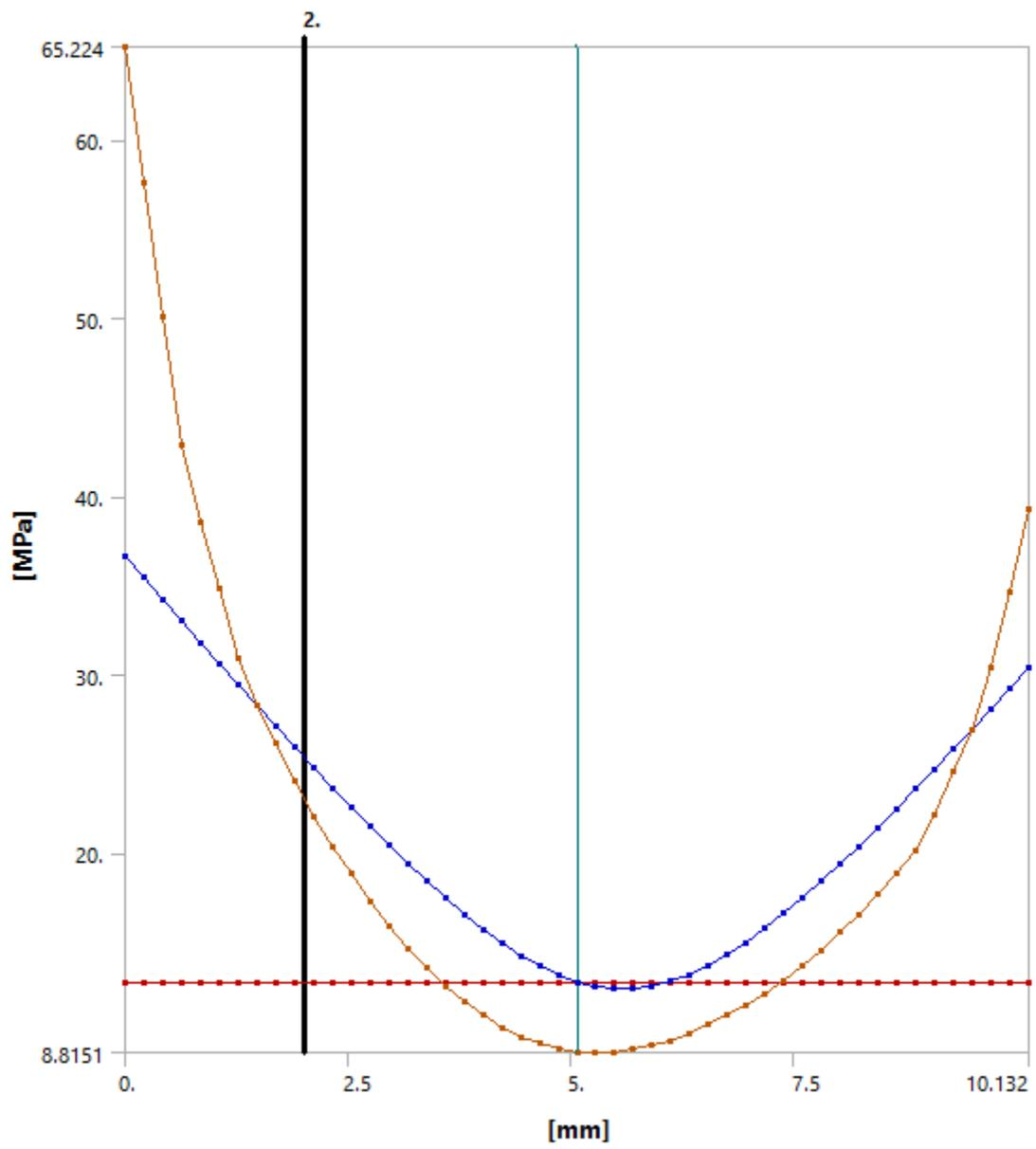
Figure 23: Variant Tile Shear Pin Linearized Stress
