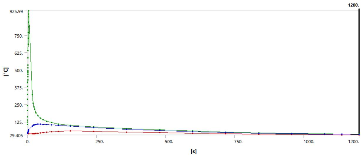
Figure 10: Transient Thermal Results for Default Tile
