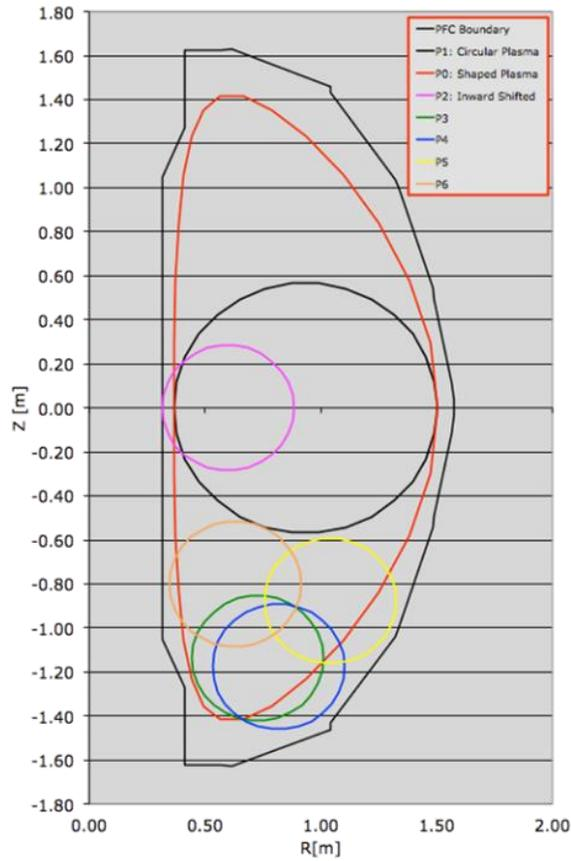
Fig. 2.1: Various plasma shapes used in the disruption simulations.
