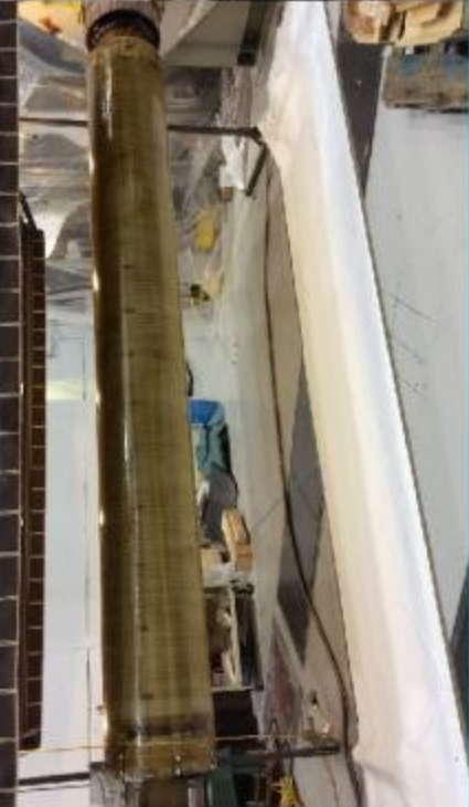
The coil was successfully VPI'd and electrically tested
