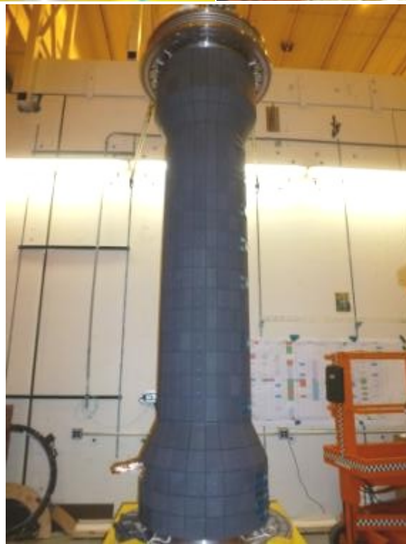
Plasma Facing Component (PFC) tiles installed on the centerstack casing
