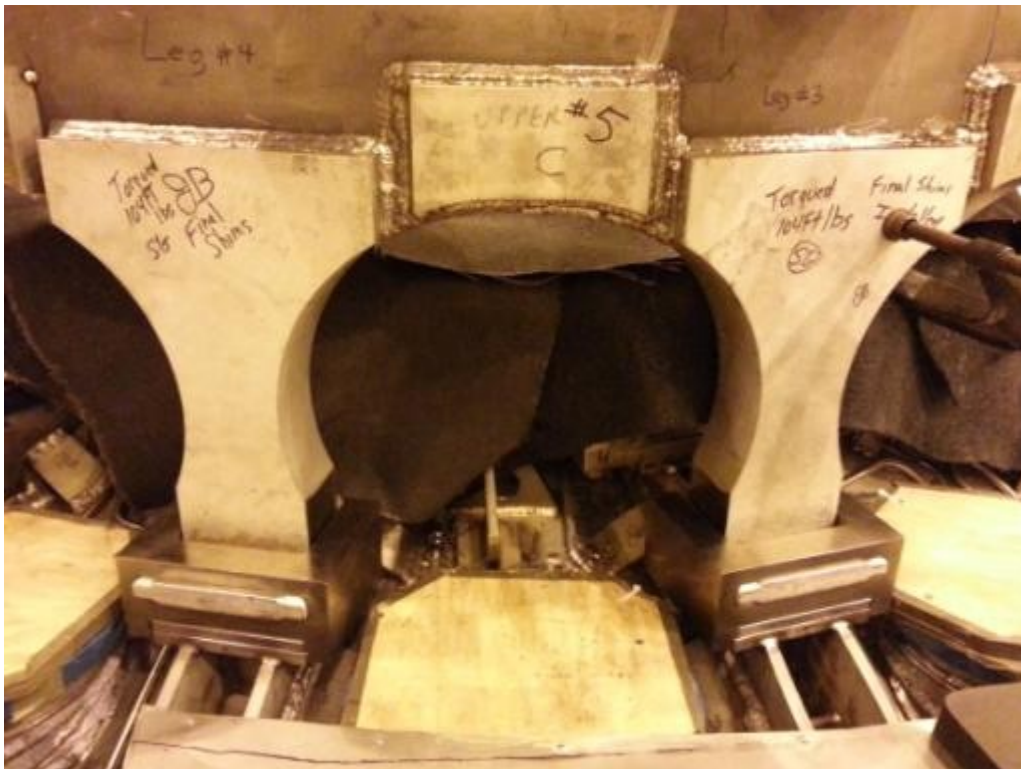
Umbrella legs upgraded from 5/8" to 2" thick
