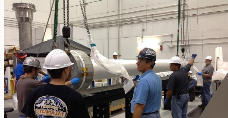
The full TF bundle is placed into a mold and VPI'd
