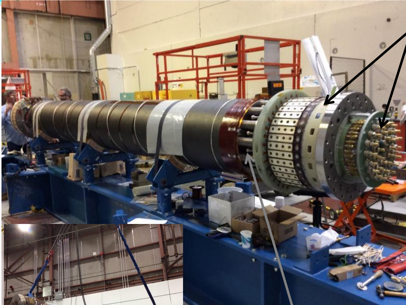
Installed Belleville pre-load system
