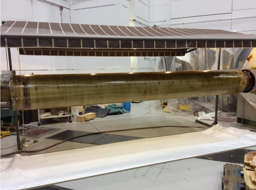
The coil was successfully VPI'd and electrically tested
