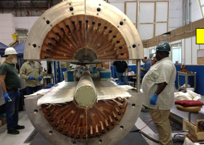
The quadrants will be assembled w/ S-2 between layers & pre-insulated G-10 core
