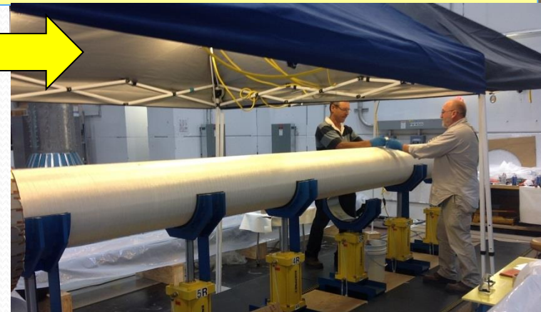
The full TF bundle is Ground wrapped with S-2 glass tape
