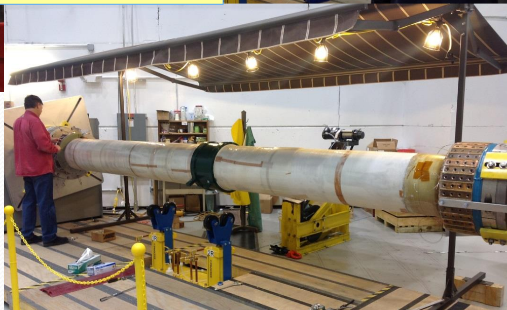
Applying Inner ground wrap insulation
