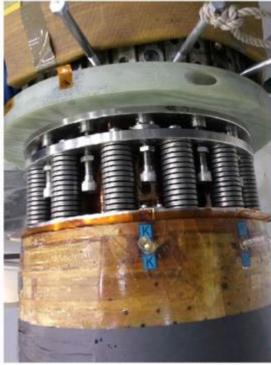
Belleville washer pre-load assembly
