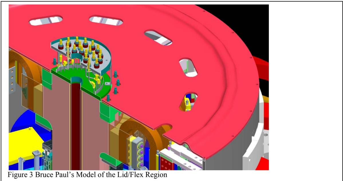
column. This is 9 mm at the elevation of the connection. The lid/flex plate is intended to bend and absorb the vertical motions elastically. Bending stresses develop at the ID and OD of the plate which produce prying moments at the bolt circles.
