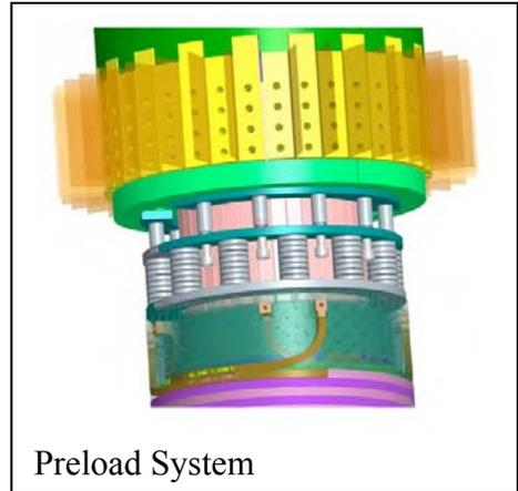
optimized to meet the requirements of the design point which has only a 9000 lb max net upward load specified for the OH coil. The system is being designed to resist a 20,000 lb "launching" load to provide some headroom for nominal loads that will be used as a basis for the DCPS set points. The faulted loading is potentially very large - 400,000 lbs. A sacrificial bumper system is being considered to mitigate the effects of the faulted loading.
