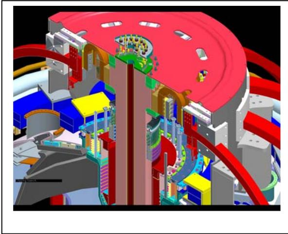
leg and the lid/or flex. They occur in the G-10 ring or collar shown as green in the figure above and labeled the crown in the figure at upper right. At the bottom of the collar, at the upper end of the TF, the teeth engage the flags of the TF legs. at the upper end of the collar, the teeth engage teeth on the lid.
