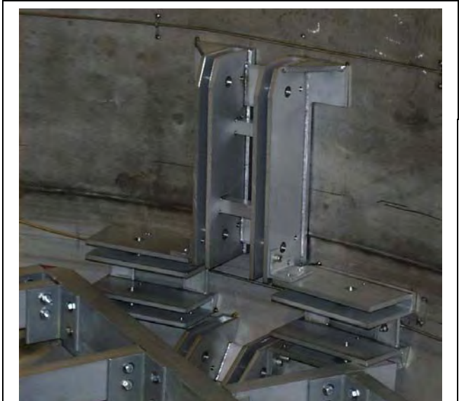
Photo of Passive Plate Attachment Details. As of November 9 the ProE model of the mounting hardware is available
