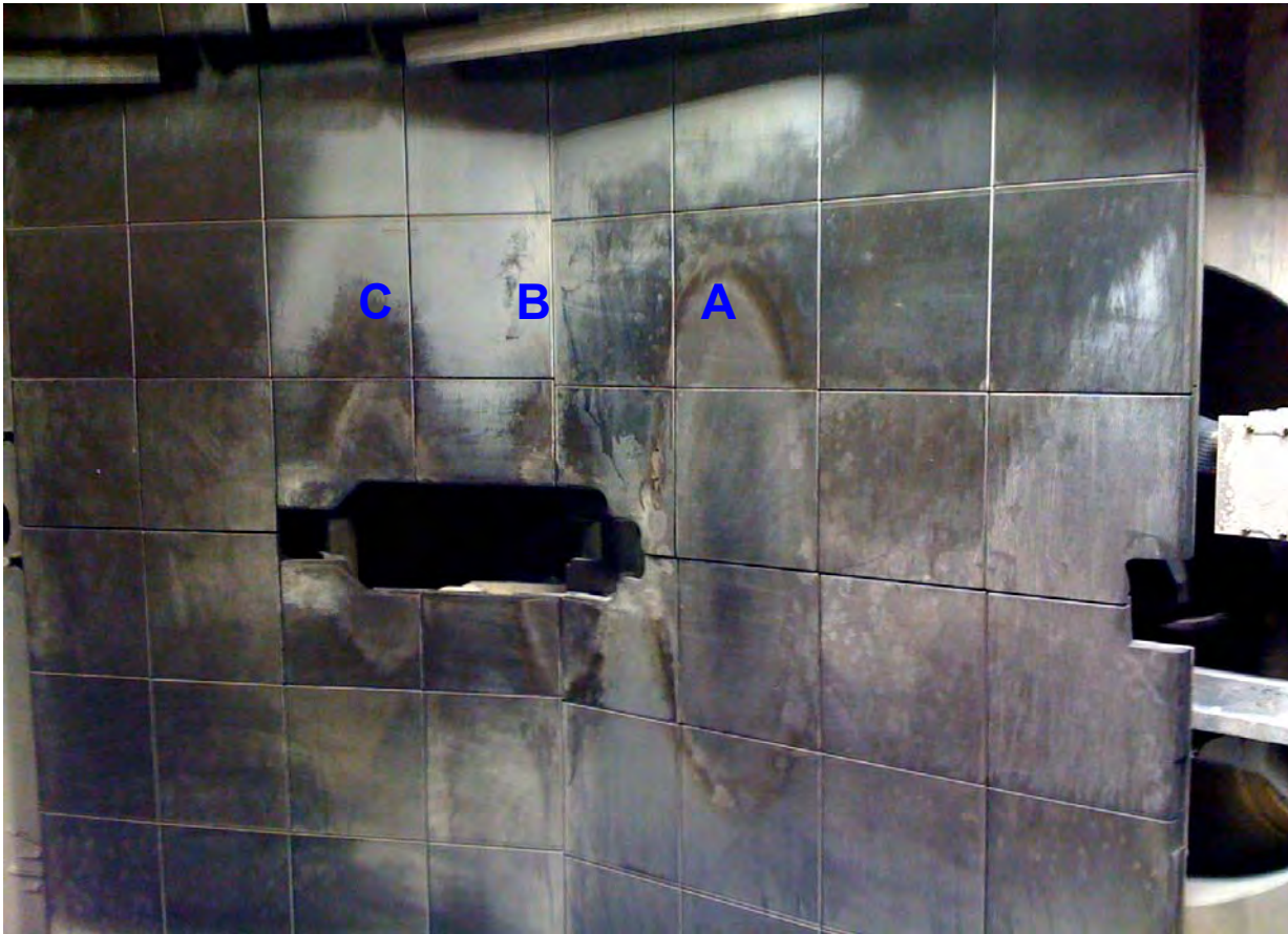
Figure 1: NSTX Armor array showing beam striping due to neutral beam sources.
