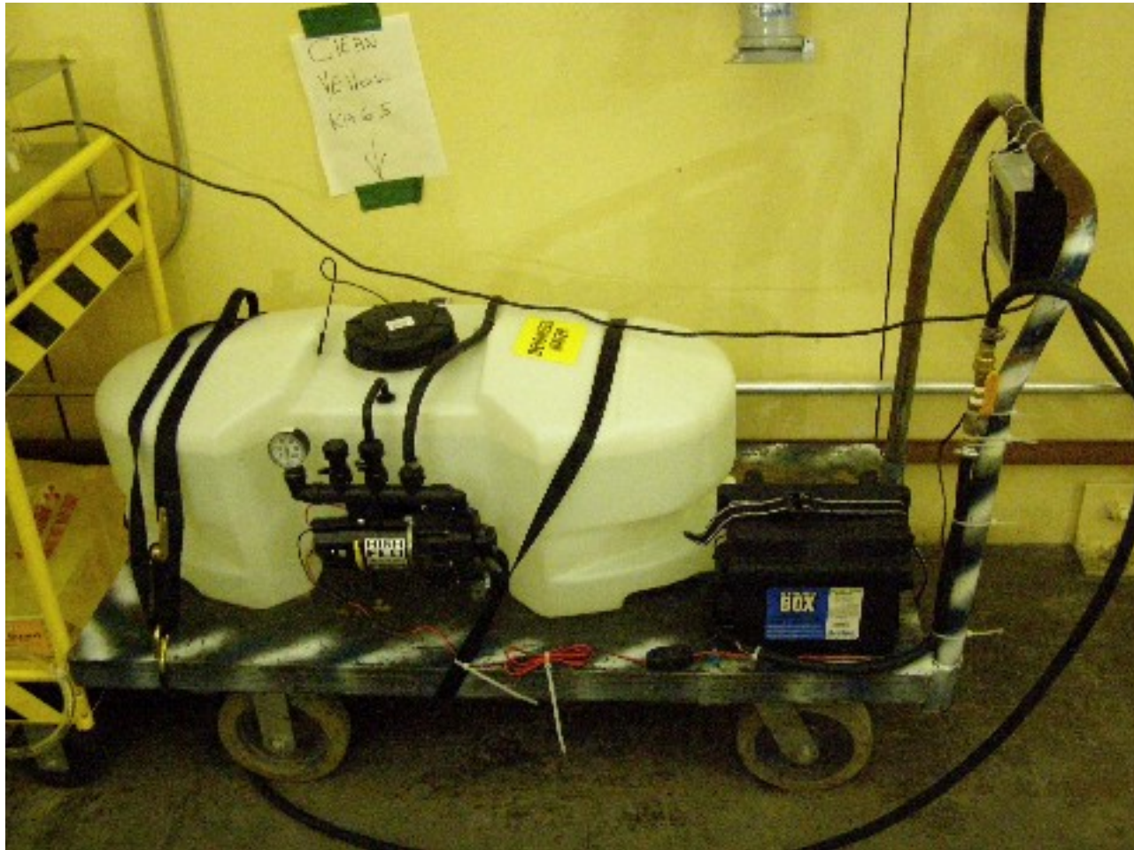
Rechargeable sprayer rig with 25 gallon DI water tank
