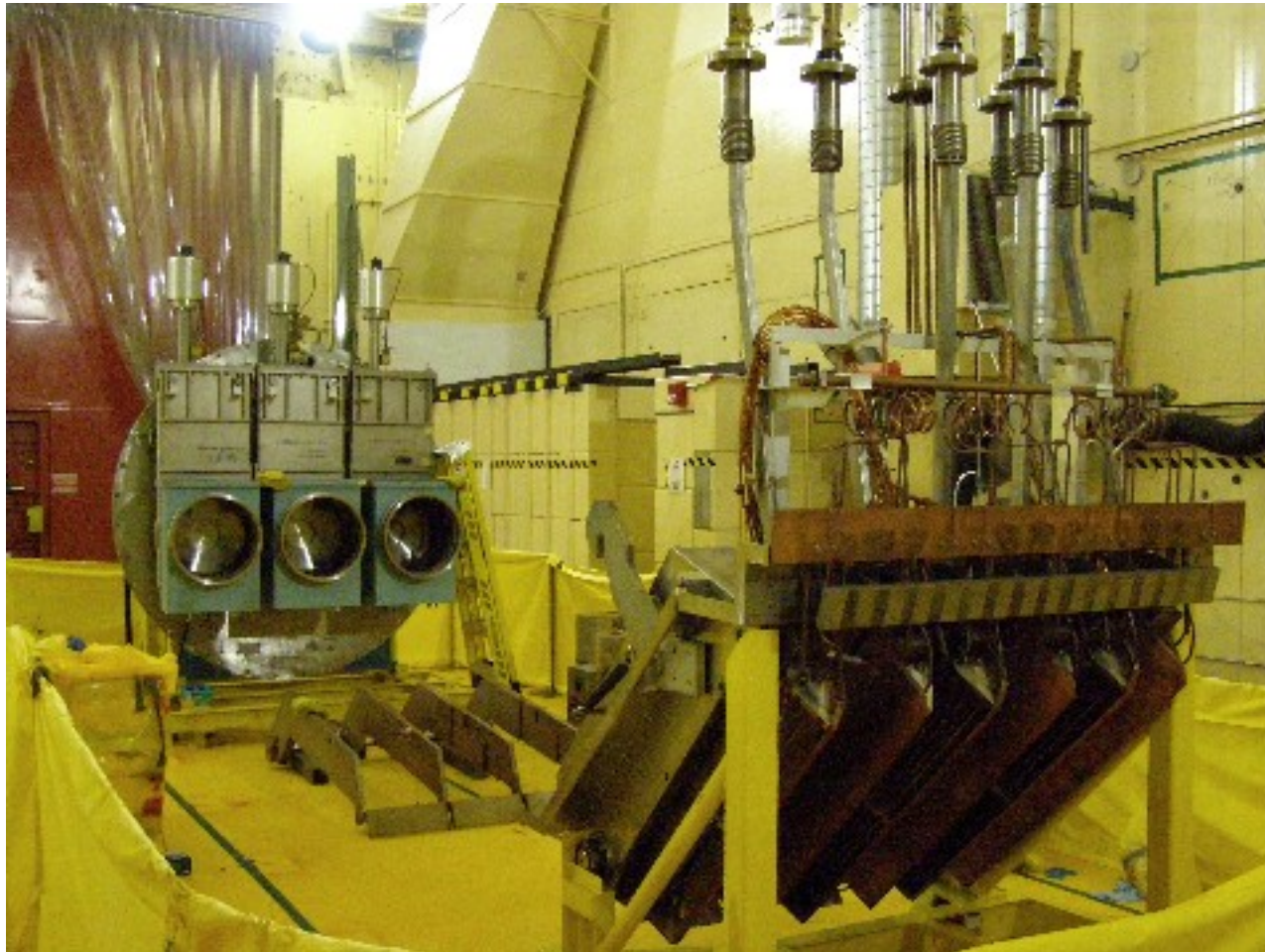
90 inch flange with OMA and SIVs, Magnet shield yoke, and Bending Magnet...
