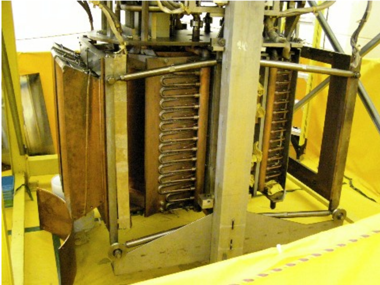
Calorimeter with shields removed for better access...
