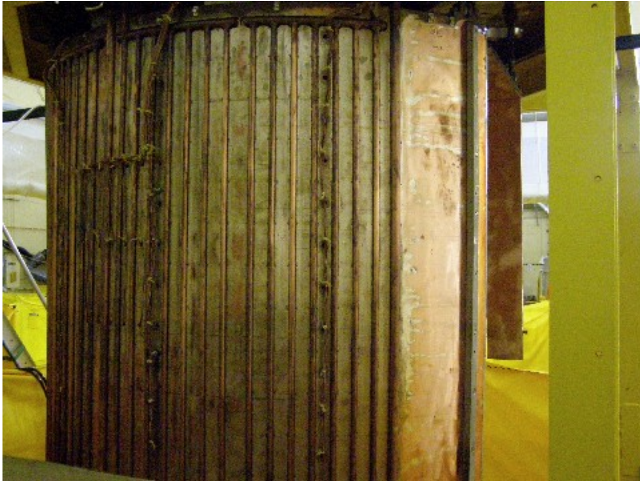
Ion dump with back shields removed for better access
