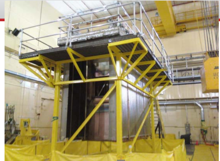
Lid and cryo panels sitting in new stand
