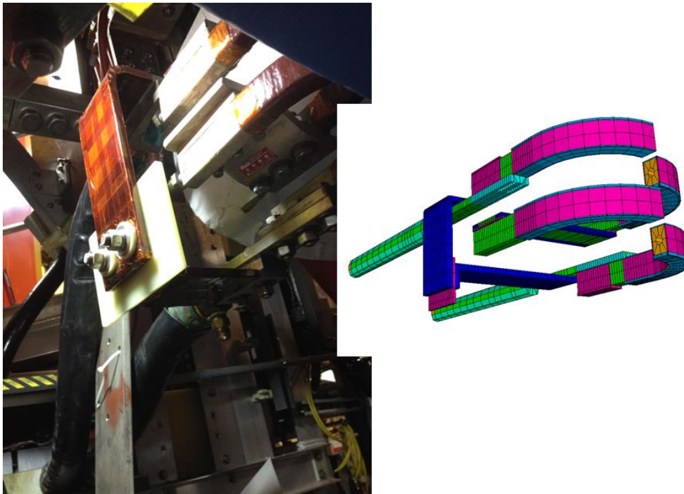
Figure 4.0-3 PF 2 /3 Terminal Reinforcements and Analysis Model Oriented as in the Photo
