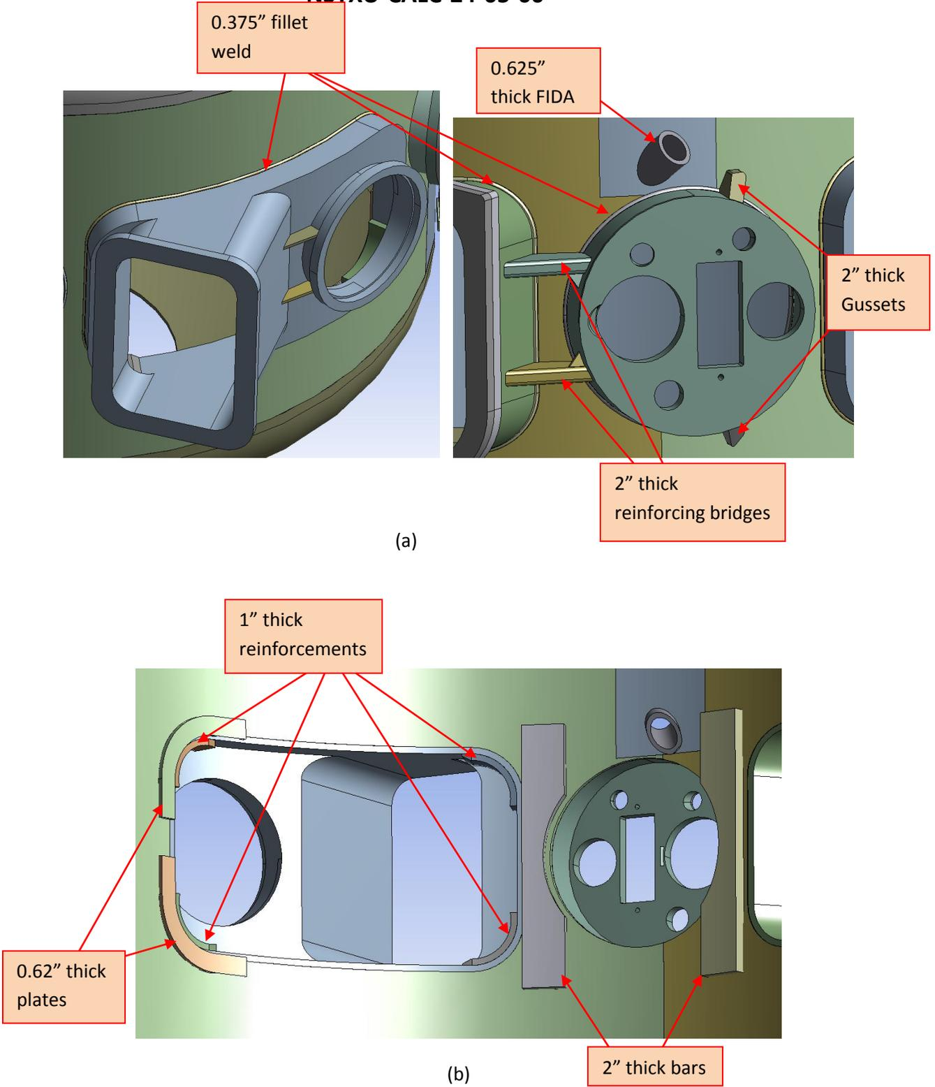
**Figure 6:** Reinforcements added: (a) on the outer body of the vessel; (b) inside the vacuum vessel
