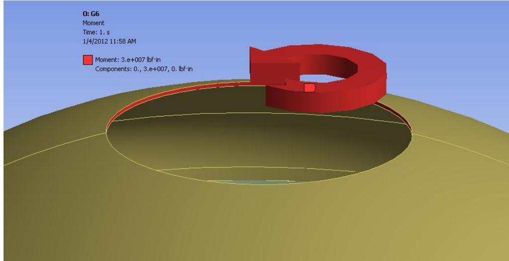
**Figure 3:** Moment due to the TF coils
