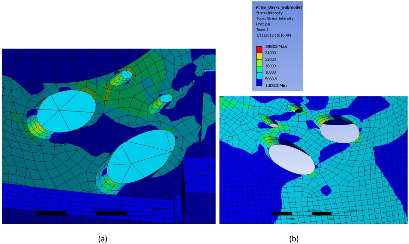
**Figure 11:** Stress results for BES diagnostics holes: (a) view from outside; (b) view from inside the vacuum vessel
