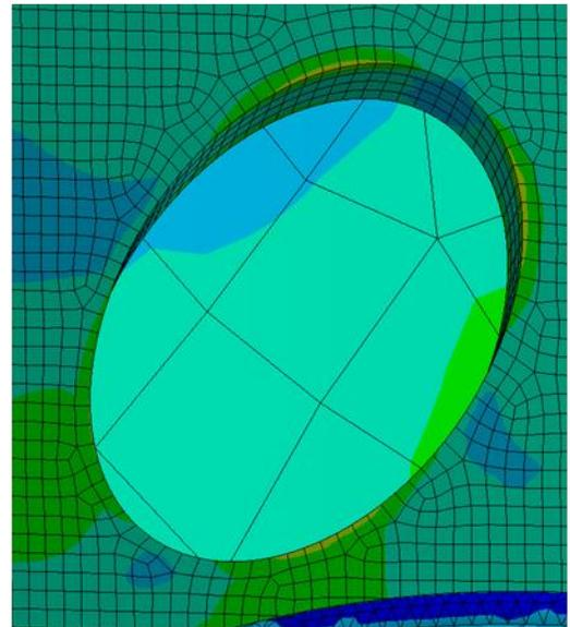
Figure 12: Stress results of the FIDA tube near Bay L
