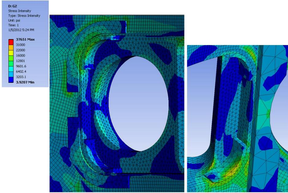
Figure 7: Global stress results around Bay K port: (a) view from outside; (b) view from inside the vacuum vessel
