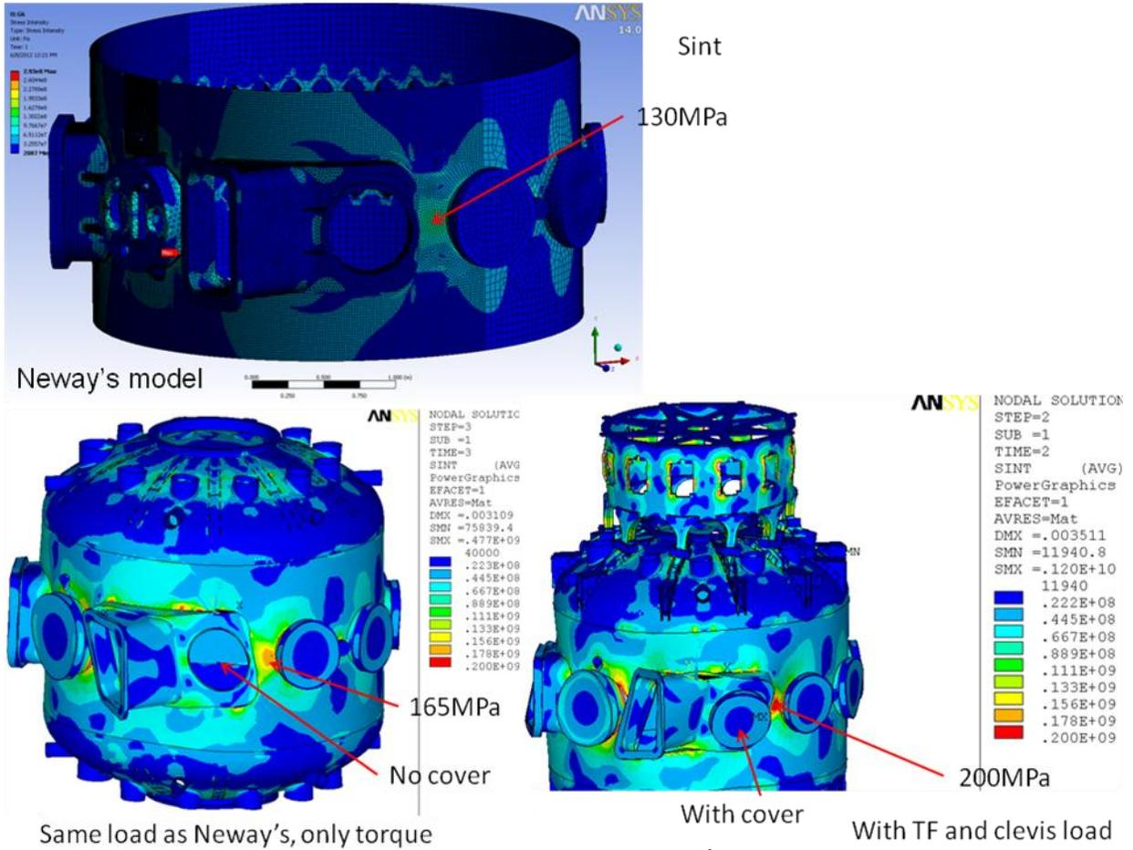
Figure 4: stress intensity around 2<sup>nd</sup> NBI port.
