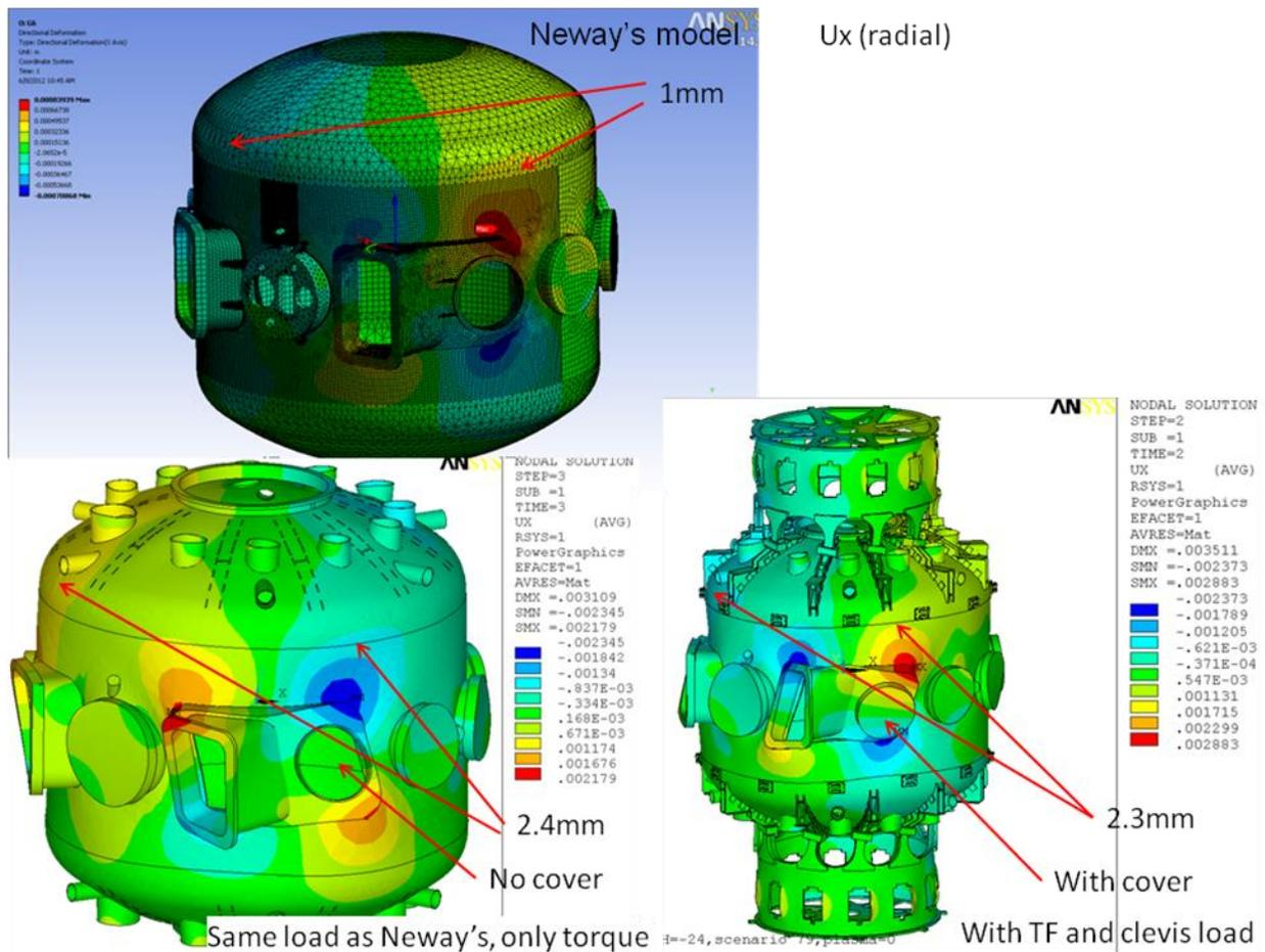
Figure 2: vessel displacement in radial direction.
