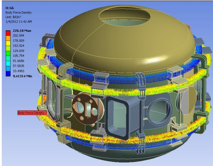
Figure 1: Electromagnetic forces in PF 4&5 Coils
