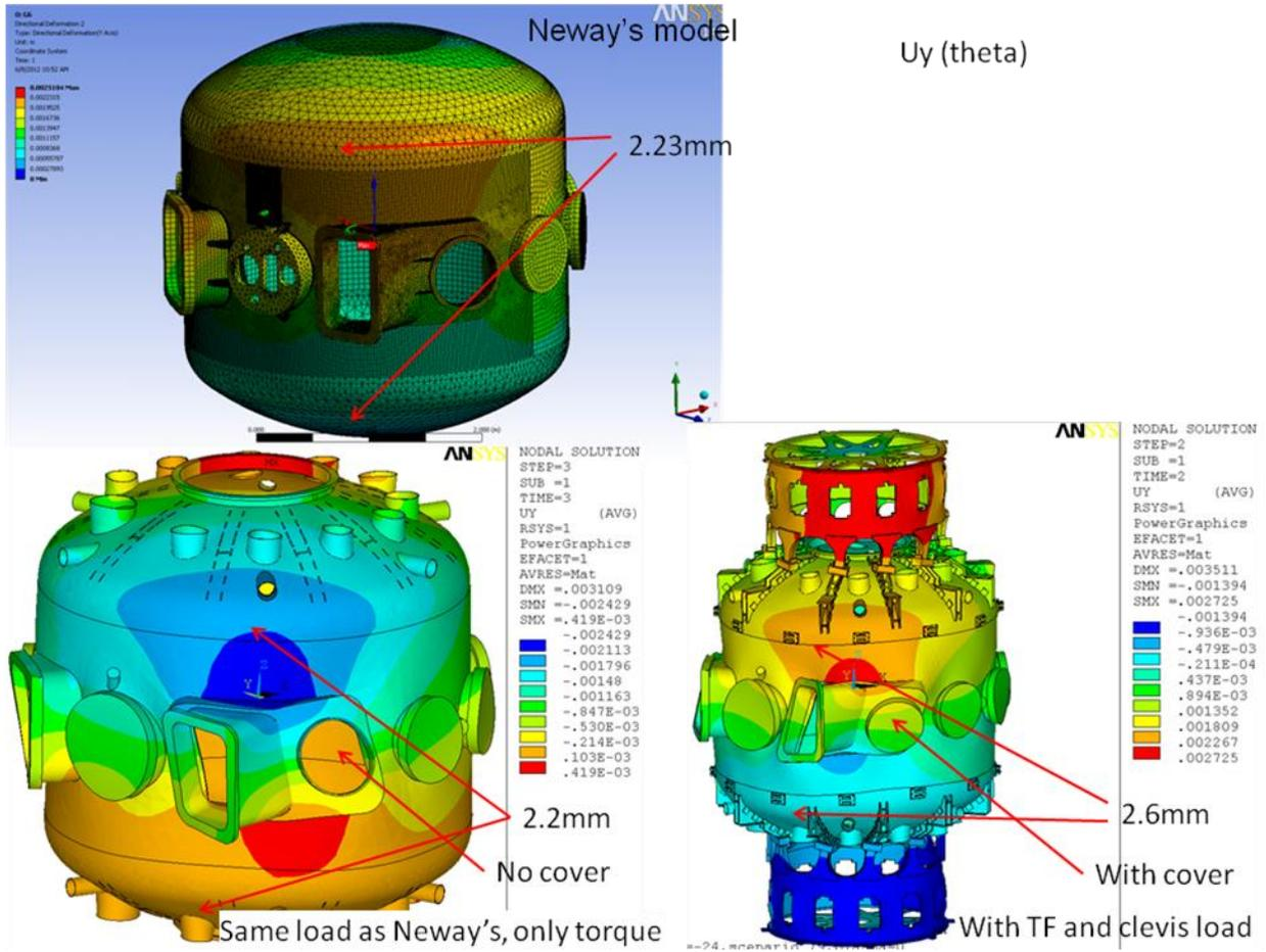
Figure 3: vessel displacement in circumferential direction.
