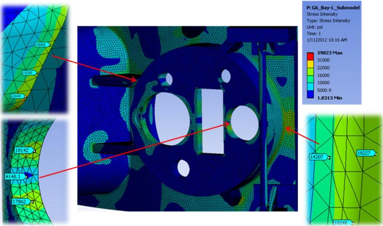
Figure 10: Sub-modeling analysis results near Bay L Port
