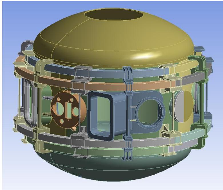
**Figure 5:** Global model of the NSTX Vacuum Vessel, PF 4&5 Coils and supports
