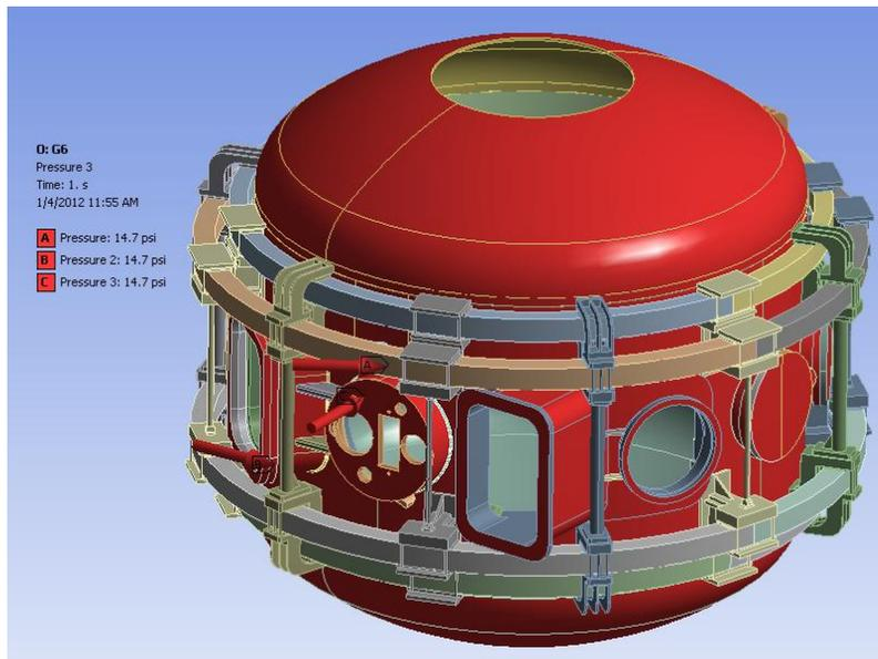
Figure 2: Vacuum pressure applied on the body of the vacuum vessel
