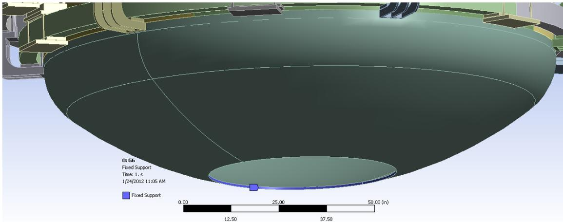
**Figure 4:** Fixed support applied to the lower dome
