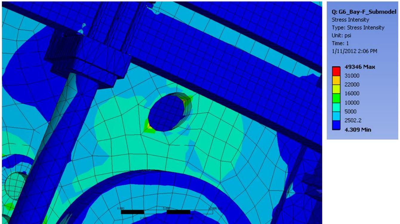
Figure 13: Stress results of the FIDA tube near Bay F
