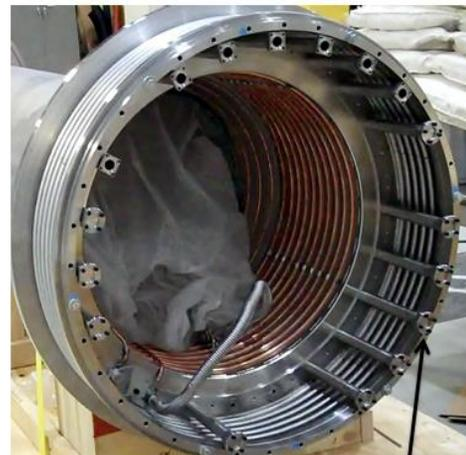
It might be possible to heat the IBDv section but it may increase the ground wrap (shim in the figure at left) above 250C
