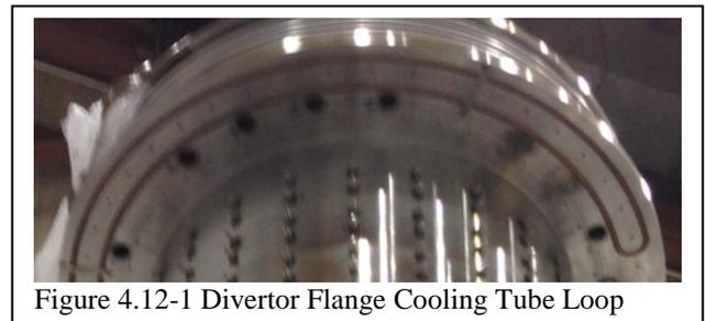
Figure 4.12-1 Divertor Flange Cooling Tube Loop
