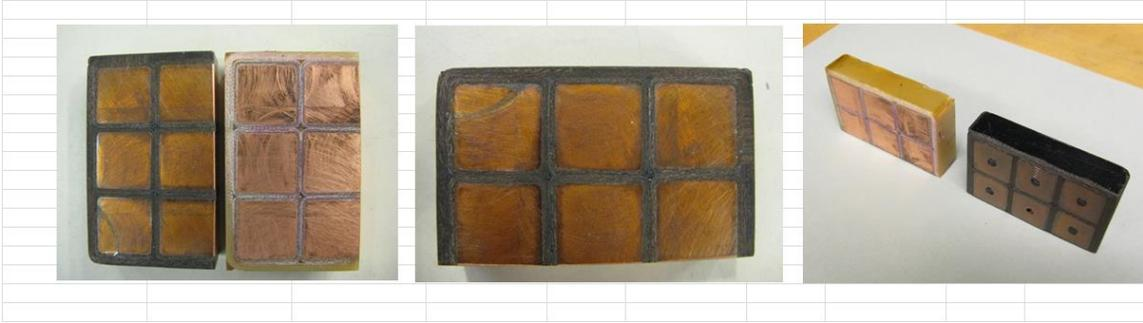
Figure 11.1.1-3-Samples “Cooked “ for 24 Hr. , Peak Temp=225C
