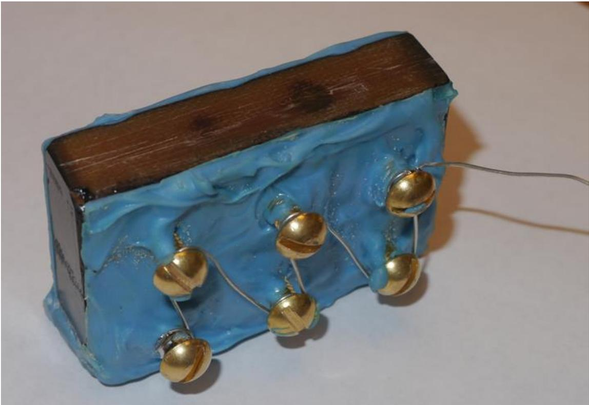
Figure 11.1.1-1 Voltage Stand-off Test Sample With Epoxy Coating to Eliminate Flash-over
