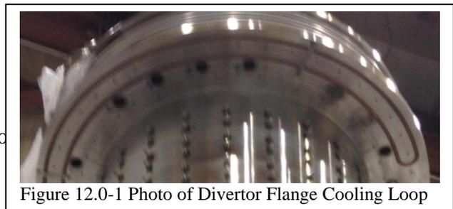
Figure 12.0-1 Photo of Divertor Flange Cooling Loop
