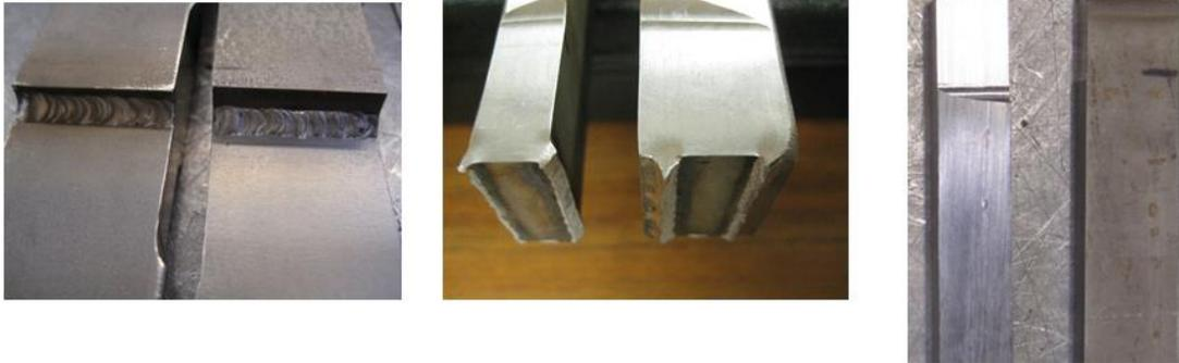
Figure 10.0-3 1/8 inch fillet weld testing
