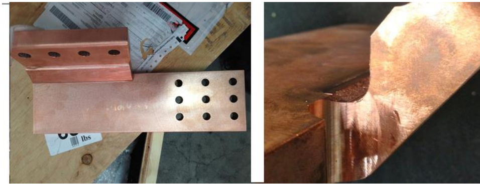
Figure 4.0-4 Flag Extension with Most Significant Loading and Radius and Relief intended to Remove Weld Root Crack
