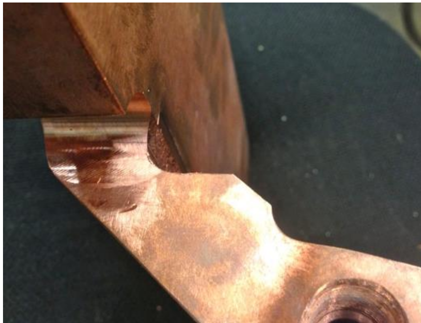
Figure 8.3.1-6 –Type “C” Weld Relief – As Machined
