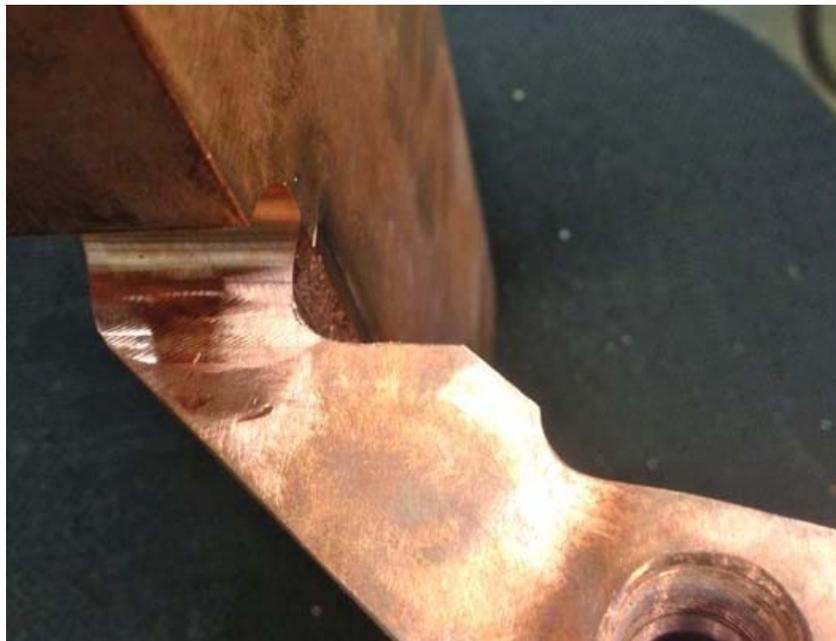
Figure 8.3.1-6 – Type “C” Weld Relief – As Machined
