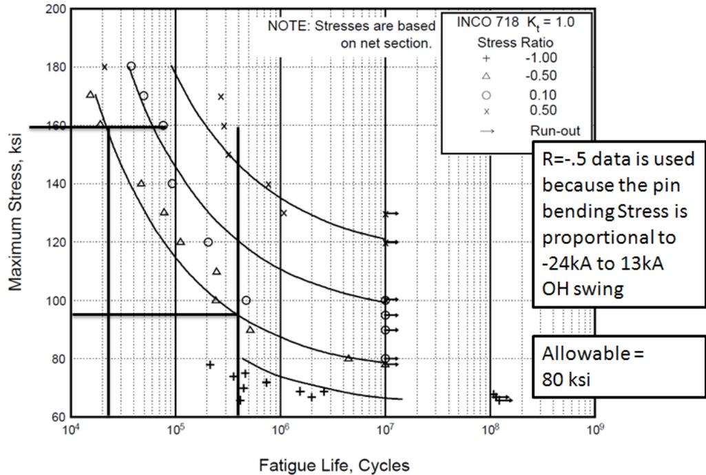
**Figure 6.3.5.1.8(f). Best-fit S/N curves for unnotched Inconel 718 bar and plate at room temperature, longitudinal direction.**
