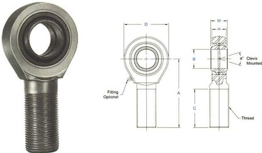
This usual configuration of a ball end exposes the thread to the cyclic loading, in the strut. To improve this the diameter of the threaded end was increased to the ID of the pipe strut.
