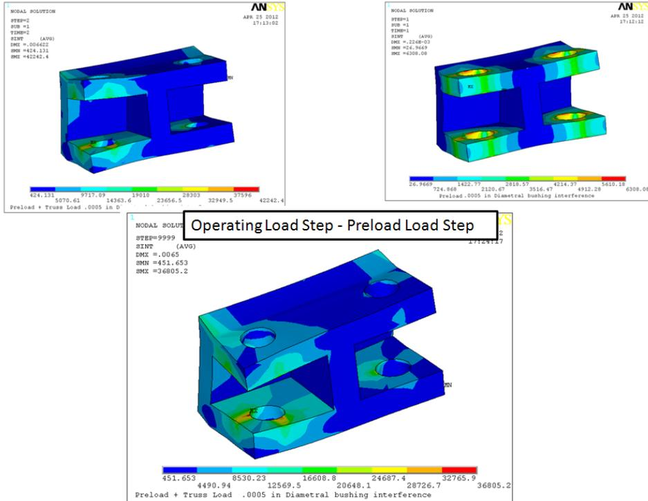
Figure 9.1-2 Clevis Plate Stresses with an interference fit.
