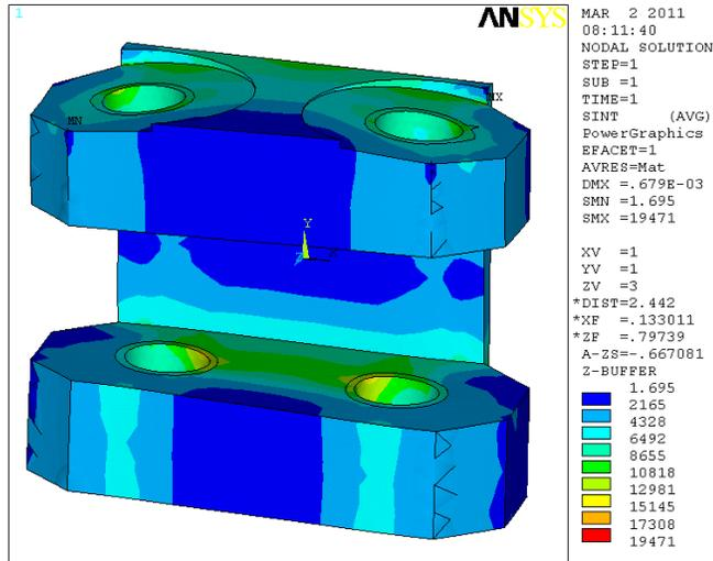
Figure 9.0-2 Figure Stresses based on a 20,000 lb Shear Load
