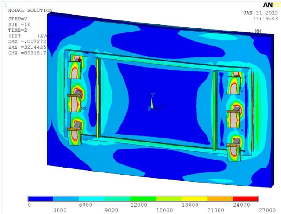
Figure 19.2-5 Stress in Vessel Wall and Weld With Contours Set at a Maximum of 27ksi
