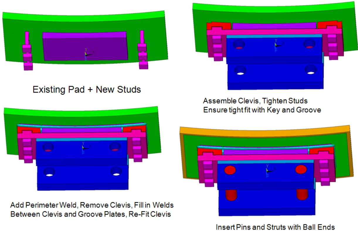
Figure 19.1-2 Bolted Clevis with Added Groove Plates
