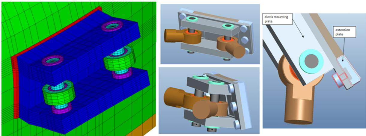
Figure 3.0-4 Clevis Details in the Late 2011(Right) and March 2012 Design (left)
