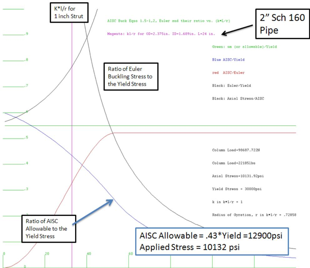
Figure 13.1-3 Qualification of 2" Sch 160 Pipe - Currently (July 13 2011) Not Chosen because the strut ends would have to have plugs welded in and a solid 2" OD rod can simply be drilled and machined to take the male spherical ball ends.
