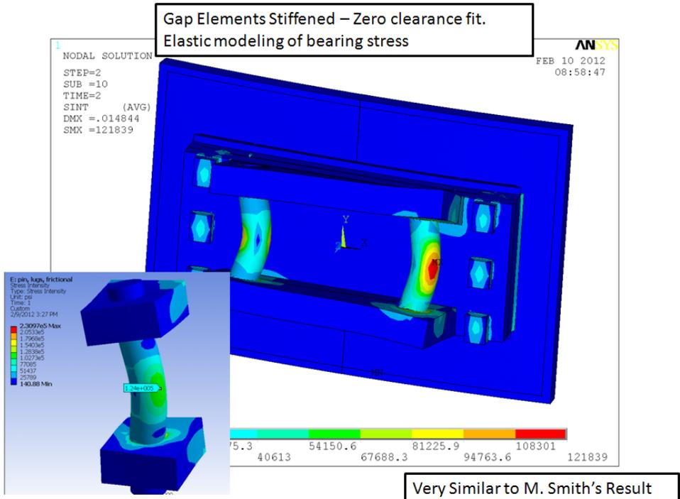
Figure 11.0-5 Study of the Effect of Pin Fit-Up
