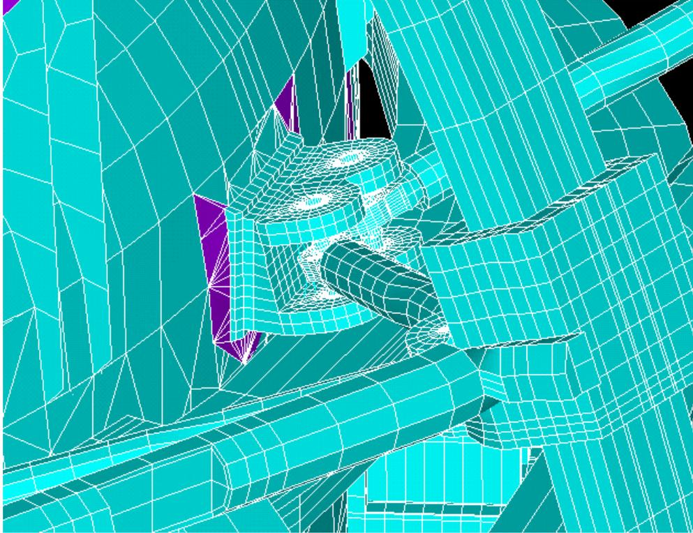
Figure 12.0-6 FEA Model/ Geometry Study to Show Clearance Issues with the Ball End
