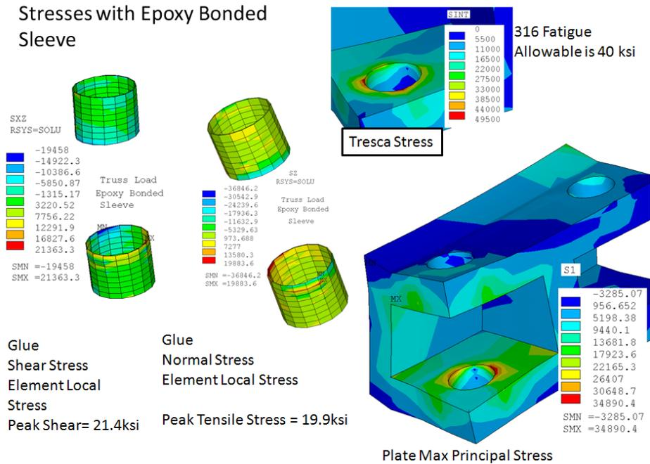
Figure 9.1-7 July 2012 Analysis with a Refined Mesh Around the Hole, and Bonded Sleeve
