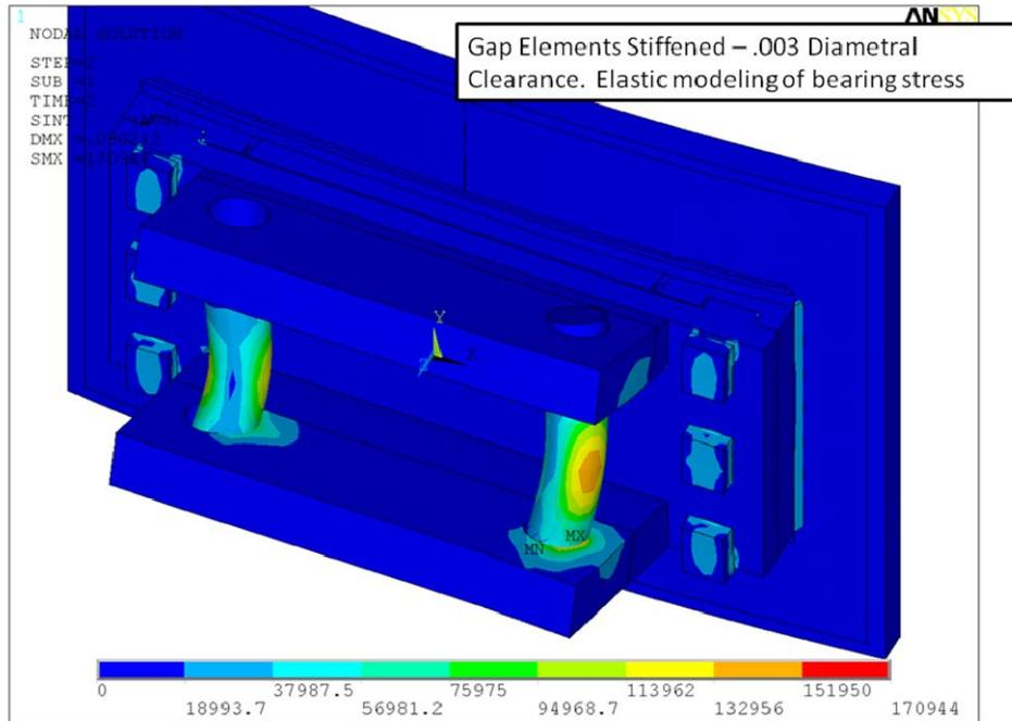
Figure 11.0-7 Study of the Effect of Pin Fit-Up (loose Fit)
