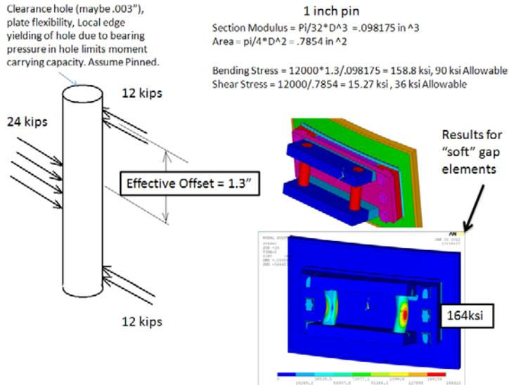
Figure 11.0-1 Clevis Pin Analysis Based on No fixity at the pin center or ends.
