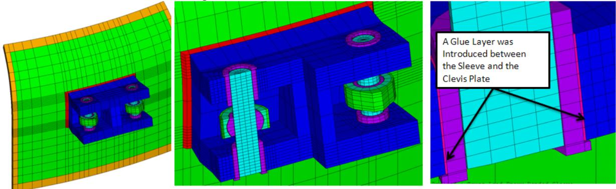
Figure 9.1-4 July 2012 Analysis with a Refined Mesh Around the Hole.
