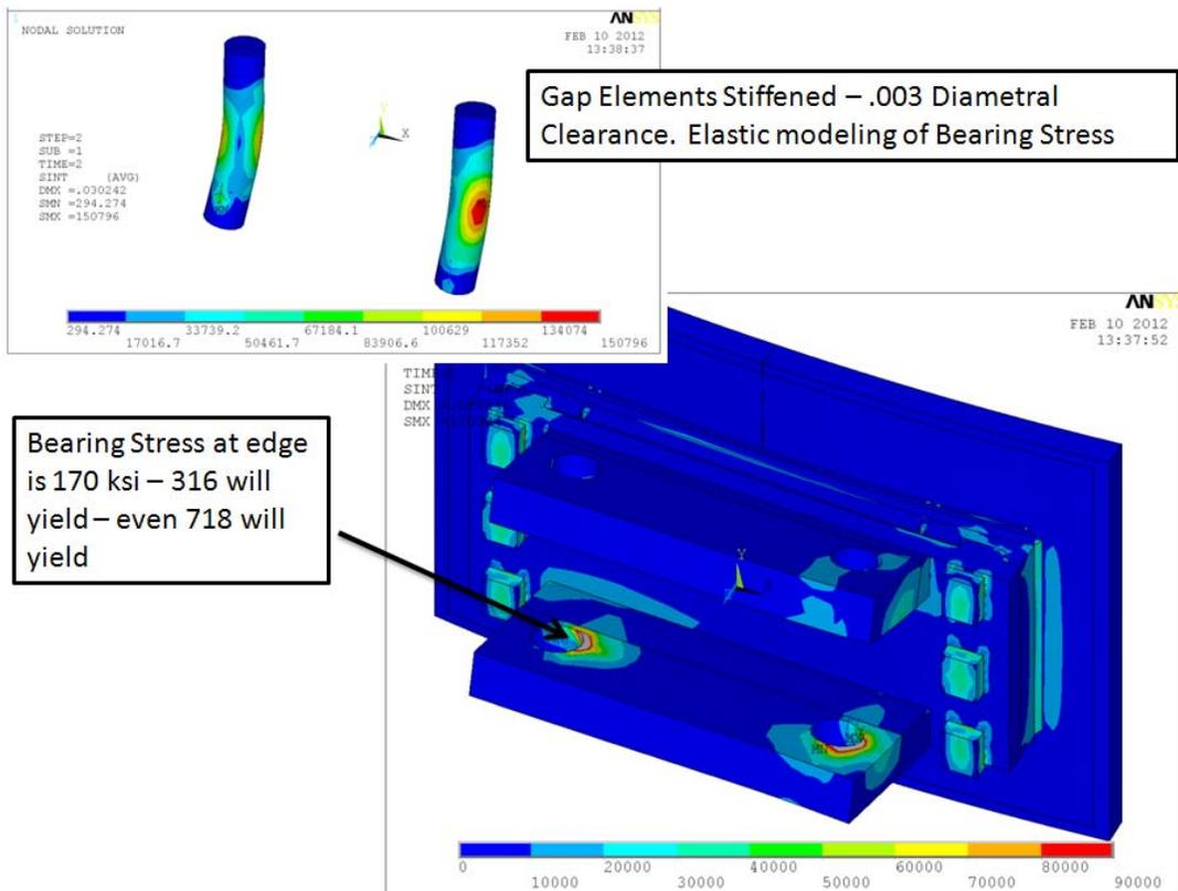
Figure 11.0-8 Study of the Effect of Pin Fit-Up (loose Fit)
