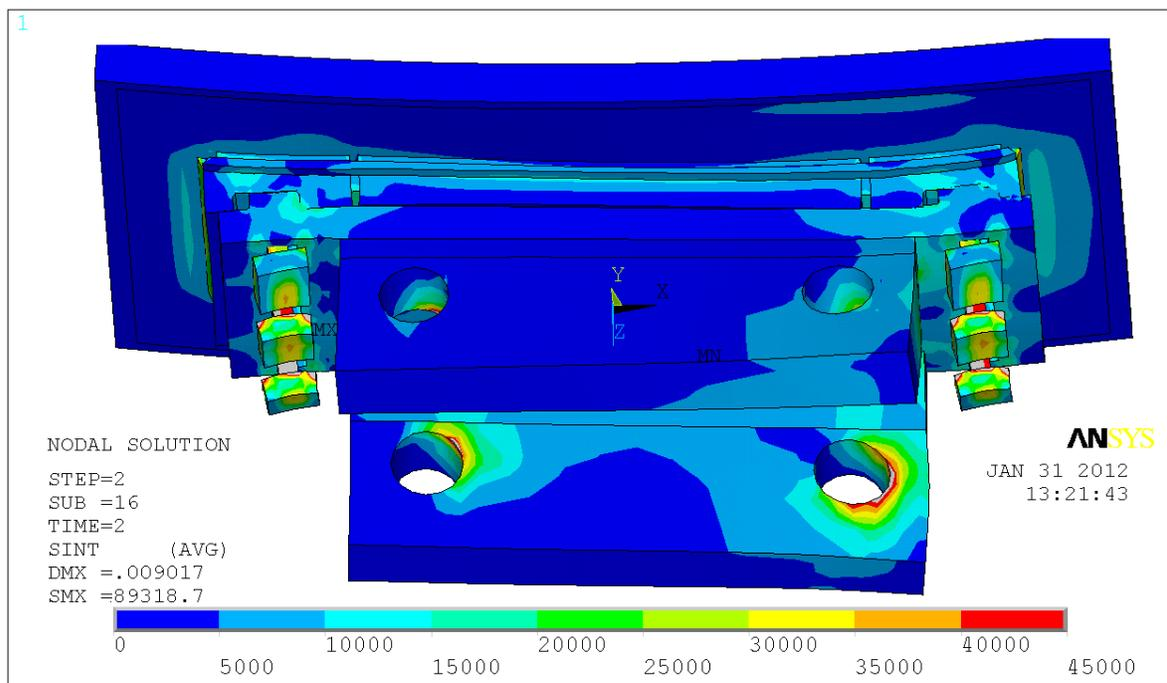
Figure 19.2-7 Stress in Vessel Wall With Contours Set at a Maximum of 45ksi
