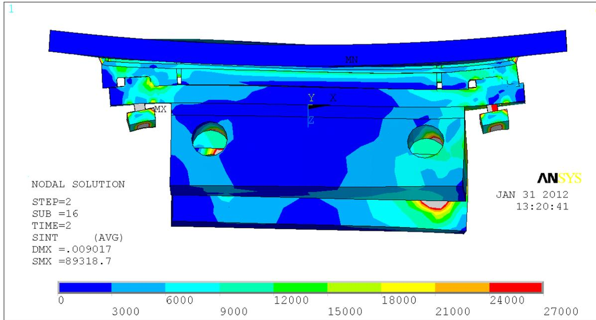
Figure 19.2-6 Stress in Vessel Wall With Contours Set at a Maximum of 27ksi
