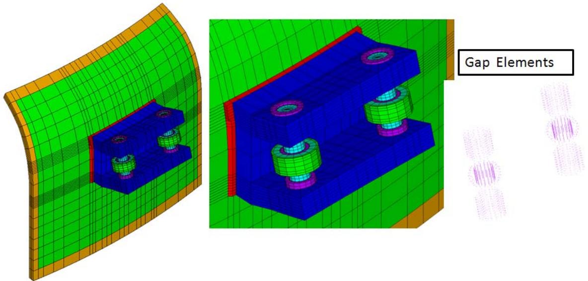
Figure 9.2-1 Model of the TF Clevis Design as of March 2 2012
