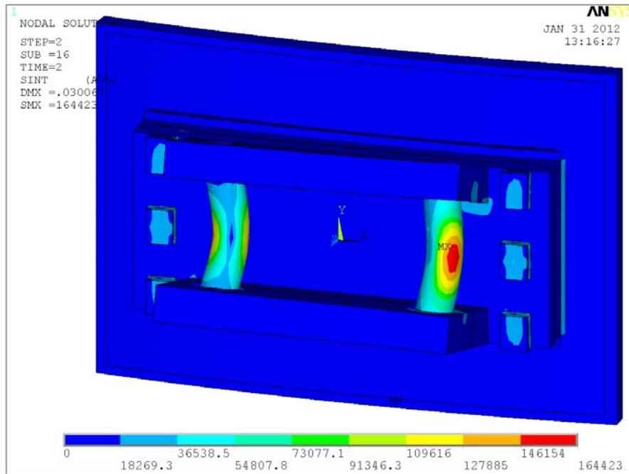
Figure 19.2-1 Bending Stress in the Pins
