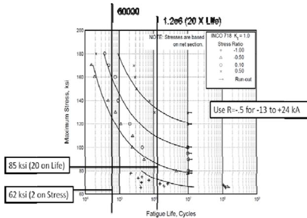
Figure 6.3.5.1.8(f). Best-fit S/N curves for unnotched Inconel 718 bar and plate at room temperature, longitudinal direction.
