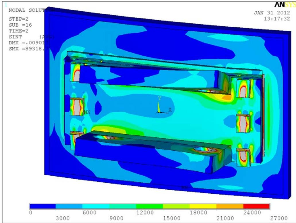
Figure 19.2-2 Stress in the Assembly with the pins Removed and the stress Contours Set at a Maximum of 27 ksi.
