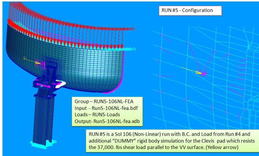
Figure 14.2-2 Special Vessel Support Bracket [10]
