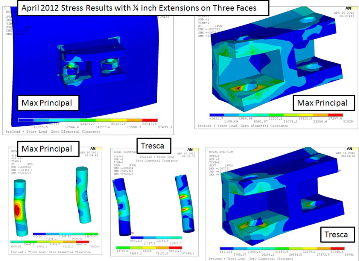
Figure 9.1-1 Clevis Plate Stress, April 2012 Geometry
