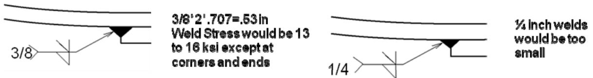
Figure 9.1-3 Clevis Weld Stress
