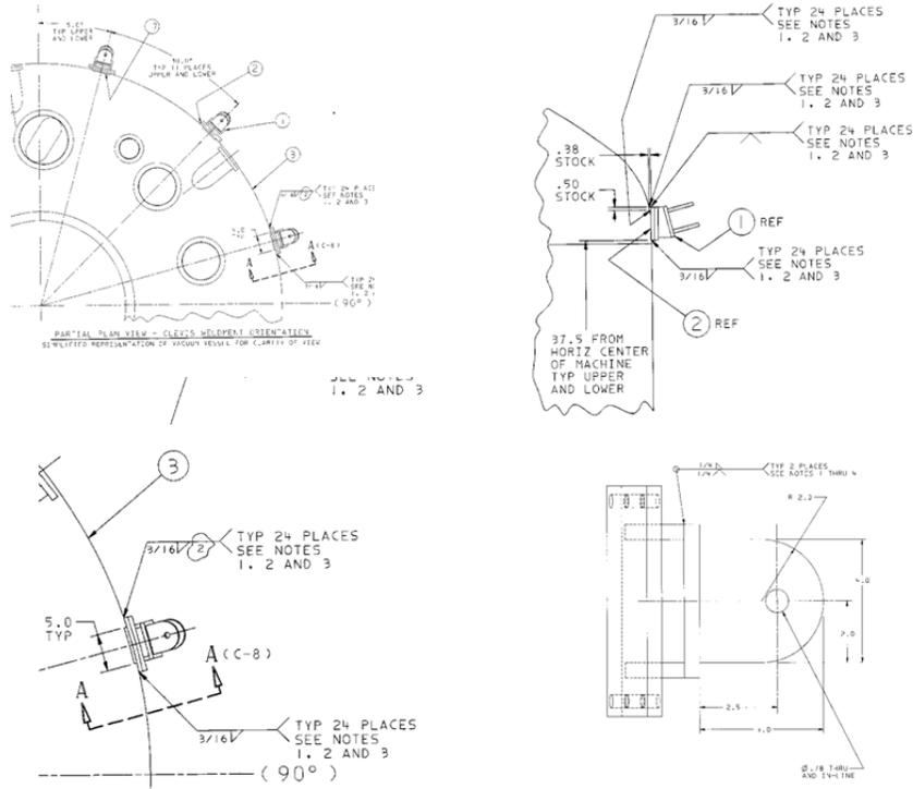
Figure 6.2-2 Clevis Details for the Original NSTX Clevis
