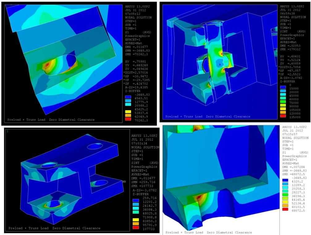
Figure 9.1-6 July 2012 Analysis with a Refined Mesh Around the Hole, and Un-bonded Sleeve
