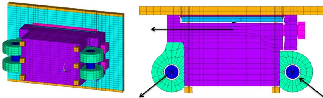
Clevis Detail with bolted edge clamp
