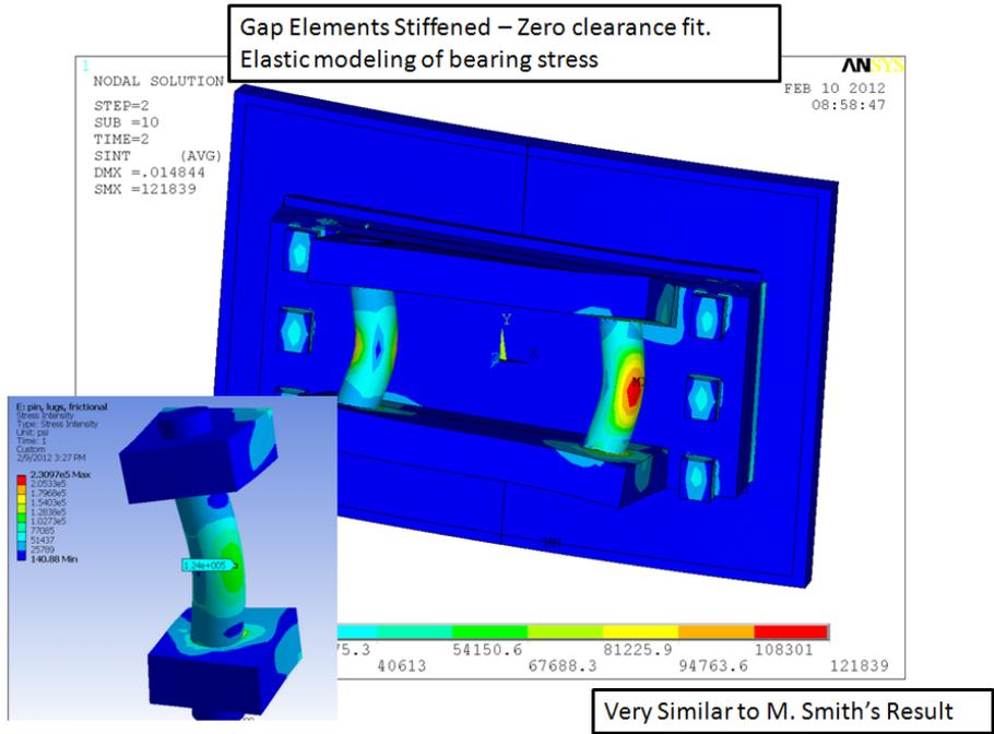
Figure 11.0-6 Study of the Effect of Pin Fit-Up
