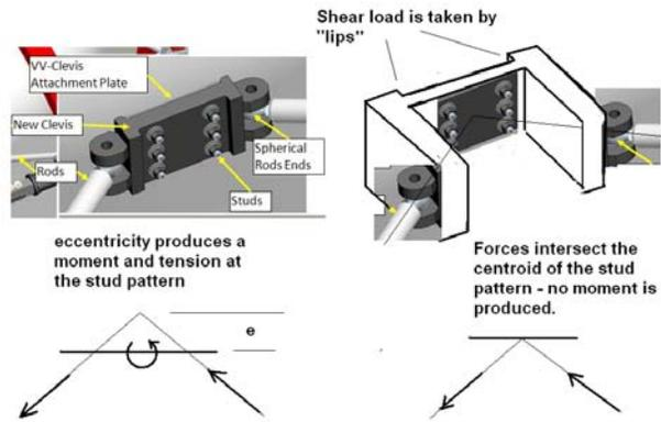
Figure 9.0-1 Mechanics and geometry that eliminates the offset moment on the clevis assembly
