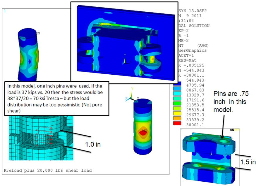
Figure 13.0-3 Clevis Pin Stress
