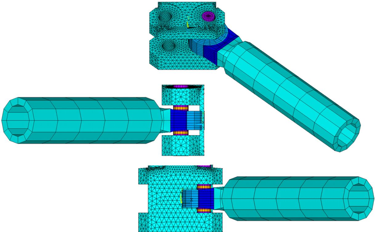
Figure 12.0-5 FEA Model/ Geometry Study to Show Clearance Issues with the Ball End
