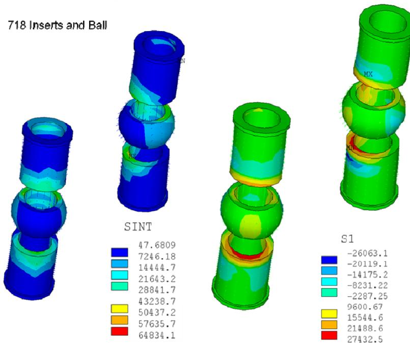
Figure 9.2-3 Bushing and Ball End Stress
