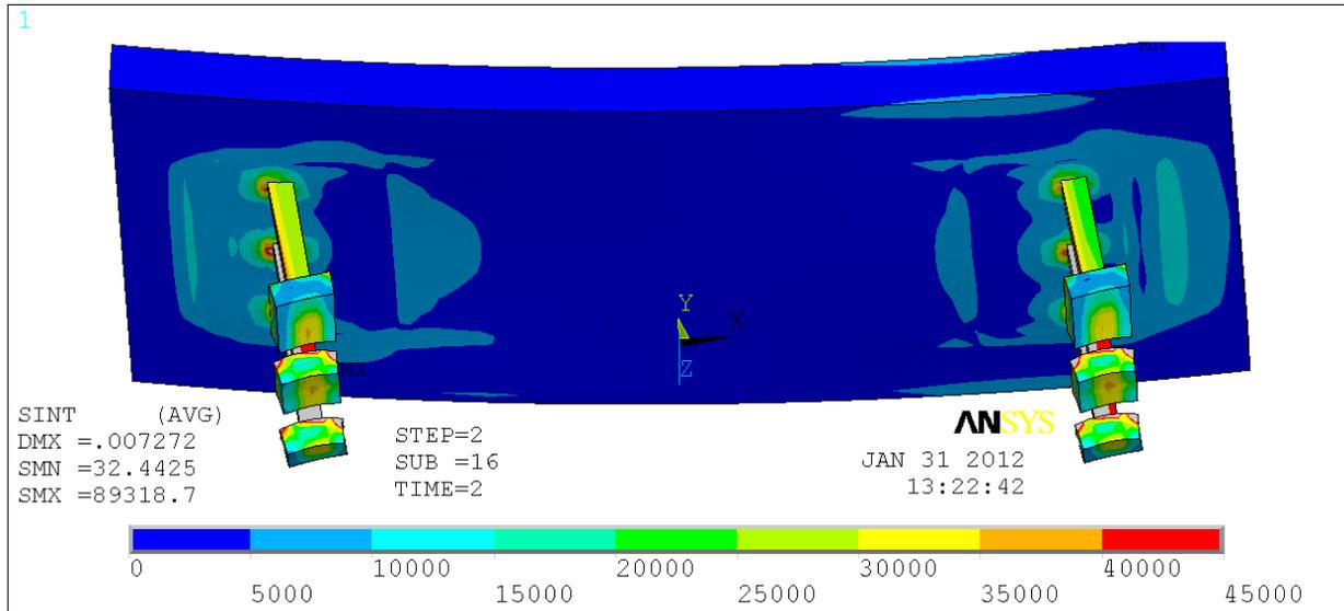
Figure 19.2-4 Stress in Vessel Wall With Contours Set at a Maximum of 45ksi, 7100 lb Stud Preload
