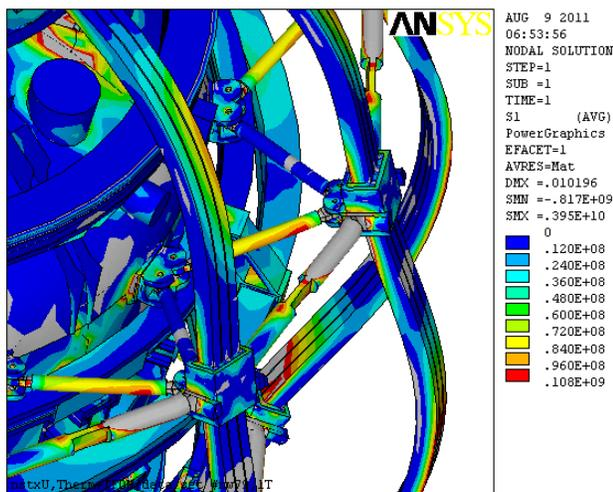
Figure 7.0-4 StrutMax Principal Stress from the Global Model[2]
