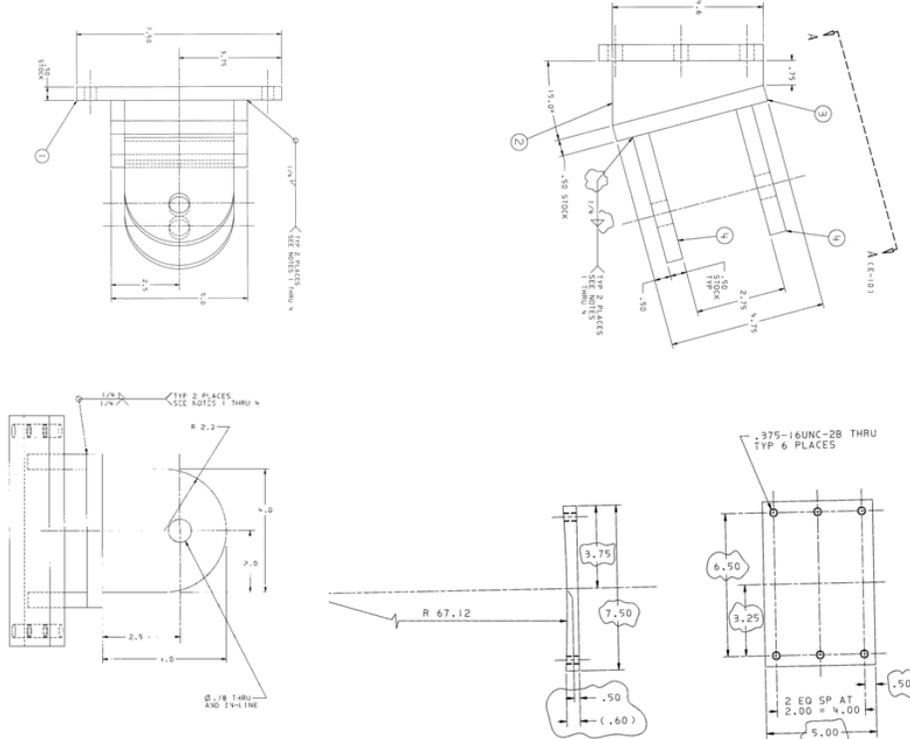
Figure 6.2-3 Clevis Details for the Original NSTX Clevis
