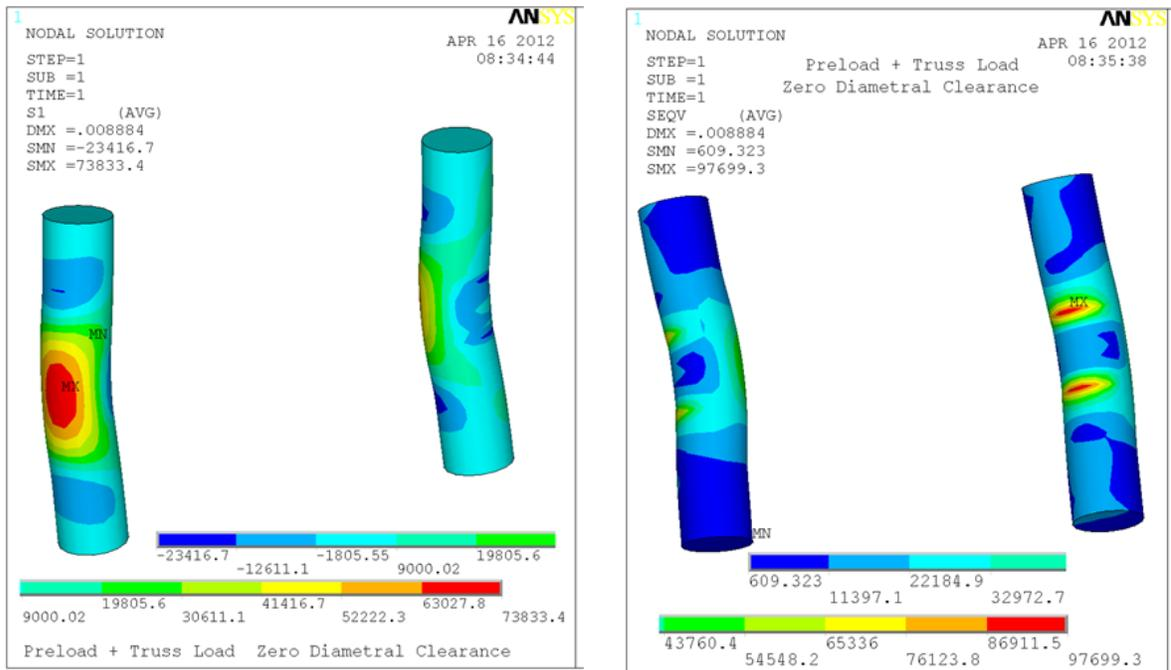
Figure 11.0-2 Clevis Pin Analysis Based on the April 2012 Clevis Configuration
