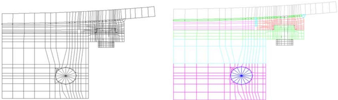
Figure 19.1-1 2D Mesh Used as the Basis for the Swept Mesh.
