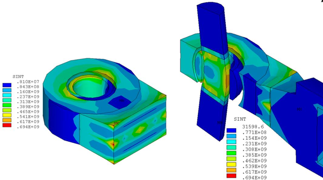
Figure 12.0-8 Analysis of the Ball End Detail
