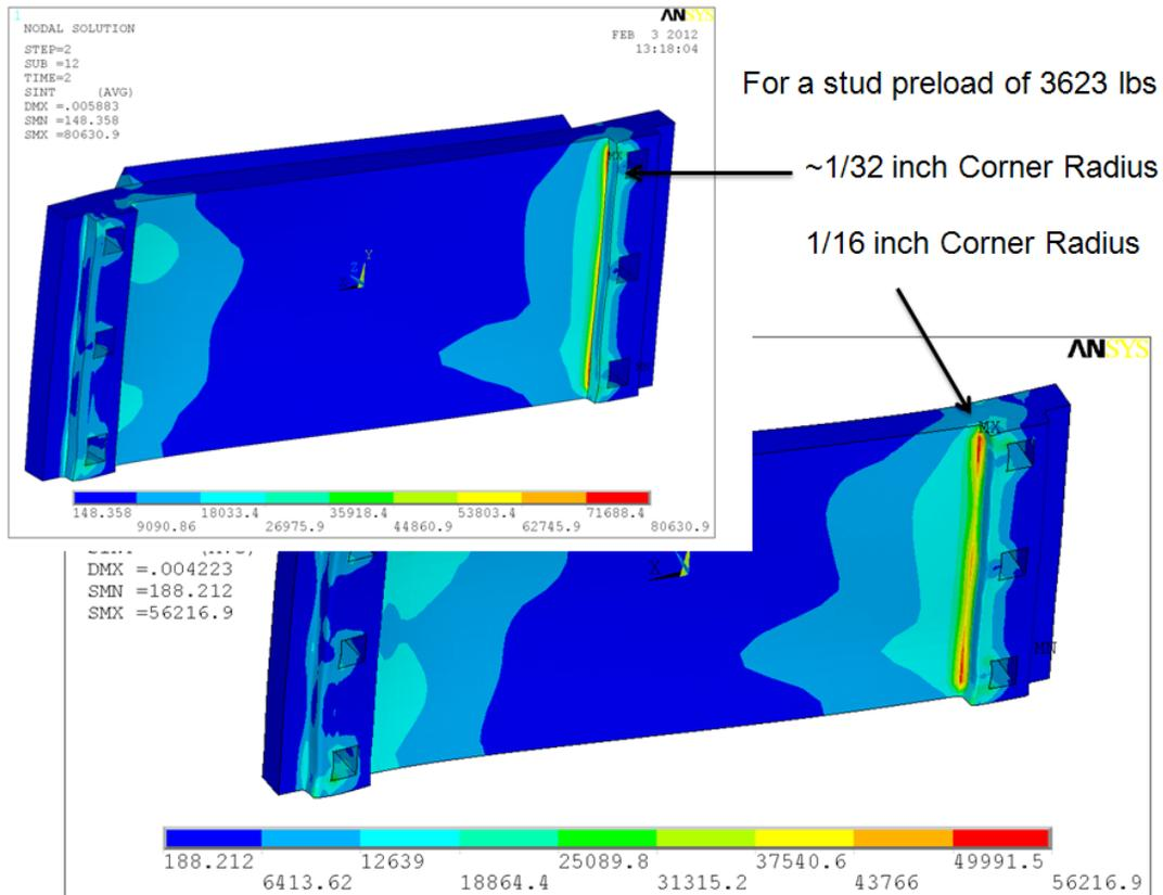
Figure 8.0-2 shows an SN Curve for 316 Stainless Steel and plots an allowable of 300 MPa or 43509 psi to satisfy the fatigue criteria. With a 1/6th radius in the tab and notch radii, the stress is acceptable for much of the height of the tab and notch. 3/23 radius would be acceptable.
