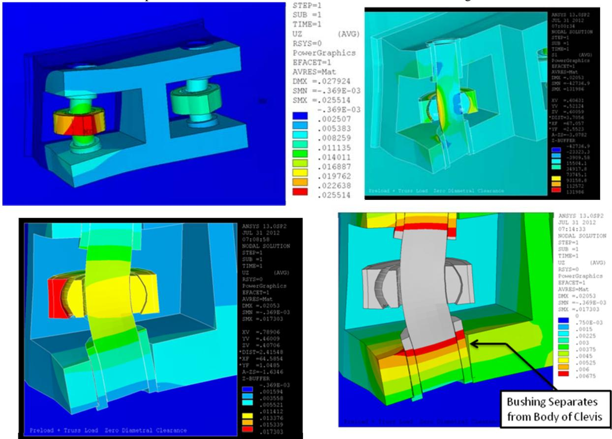
Figure 9.1-5 July 2012 Analysis with a Refined Mesh Around the Hole, and Un-bonded Sleeve
