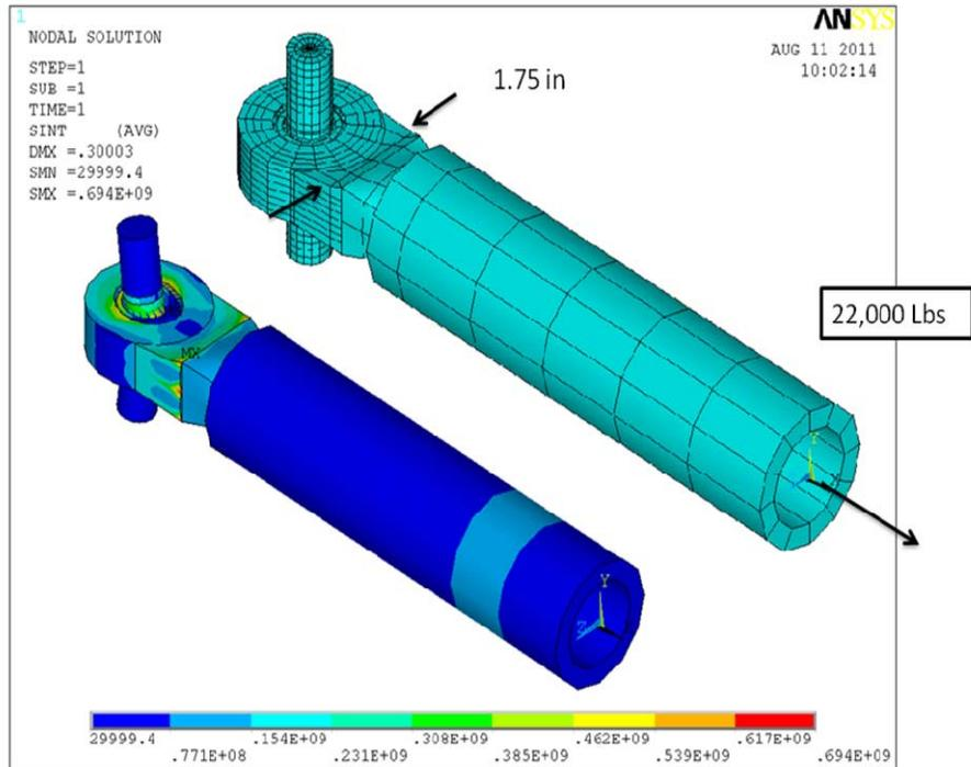
Figure 12.0-7 Analysis of the Ball End Detail
