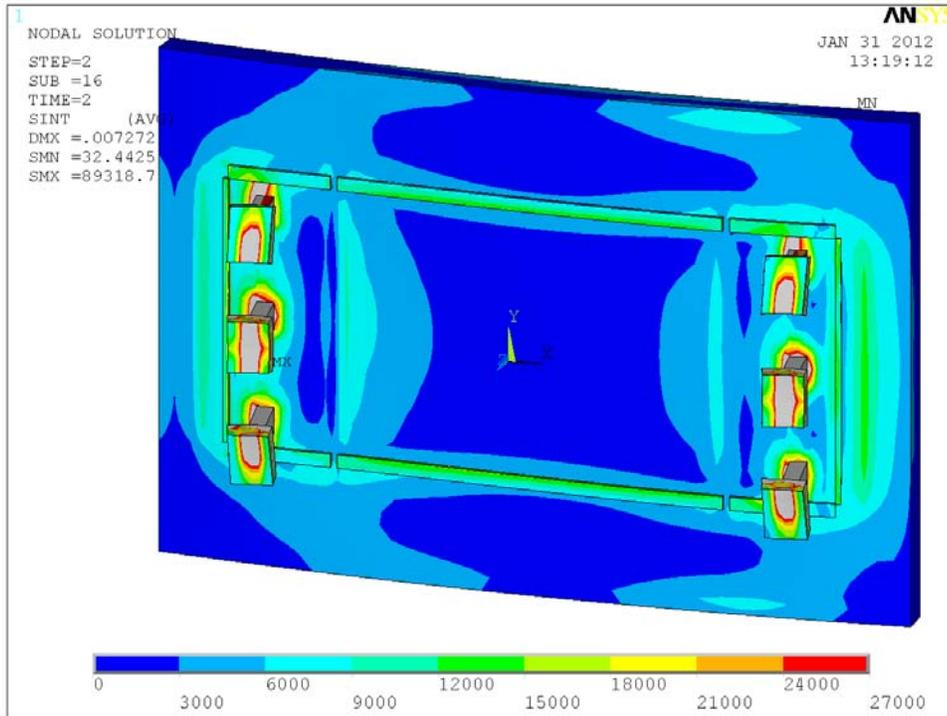
Figure 19.2-4 Stress in Vessel Wall and Weld With Contours Set at a Maximum of 27ksi
