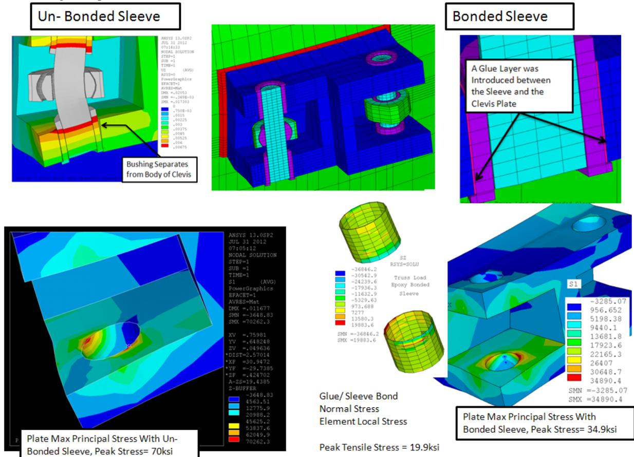
Figure 3.0-1 April 2012 Design, July Analysis Bonded and U-Bonded Sleeve
