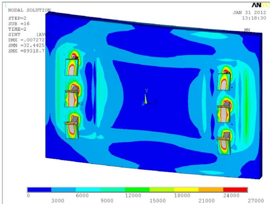
Figure 19.2-3 Stress in Vessel Wall With Contours Set at a Maximum of 27ksi
