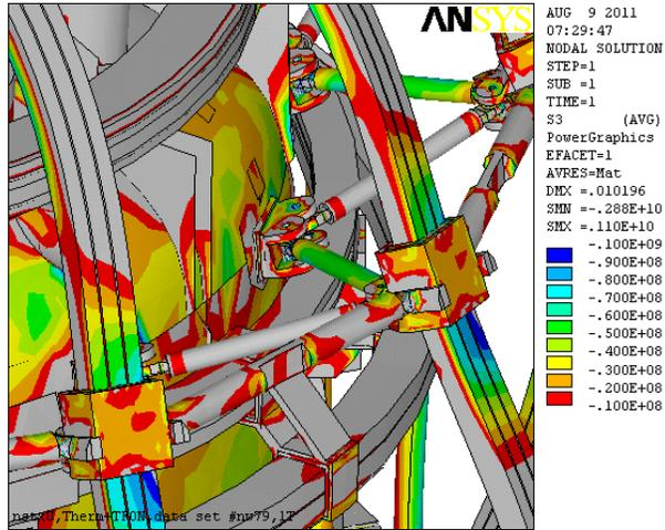
Figure 7.0-4 Strut Min Principal Stress from the Global Model[2]
