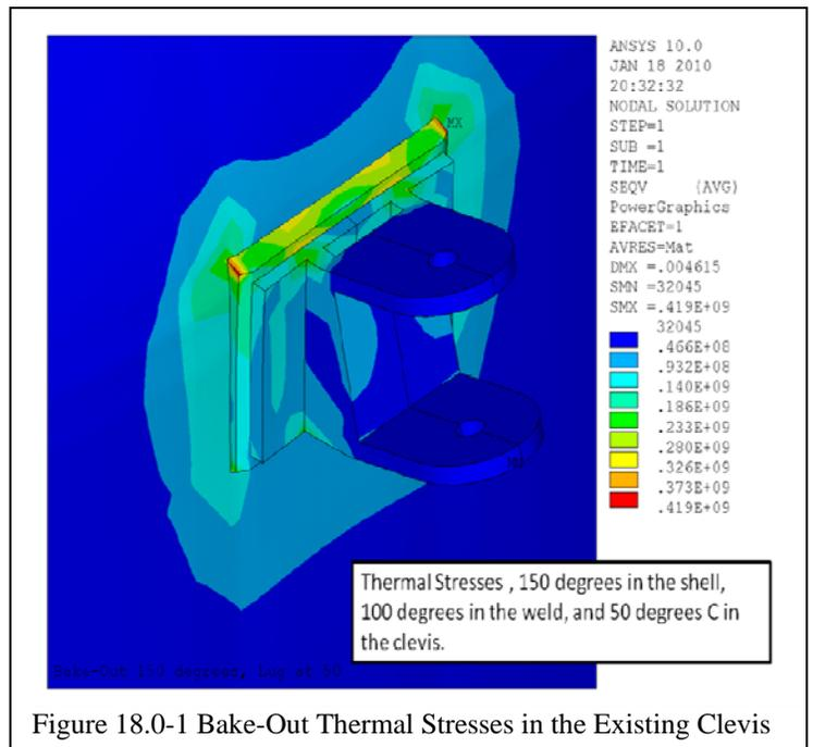
Figure 18.0-1 Bake-Out Thermal Stresses in the Existing Clevis
