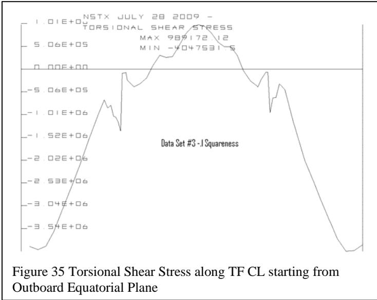
Figure 35 Torsional Shear Stress along TF CL starting from Outboard Equatorial Plane
