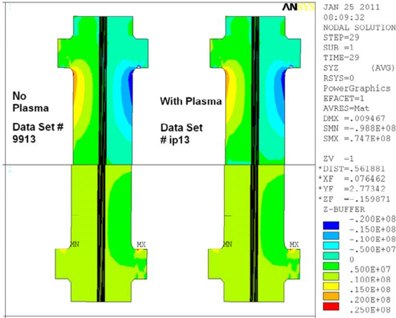
Figure 2 This shows one current set from the global model analysis, in which the plasma current effect on the torsional shear is difficult to discern. From the influence coefficient calculations it is about a 1 MPa effect (see Figure 6). The magnitude is close to 20 MPa.
