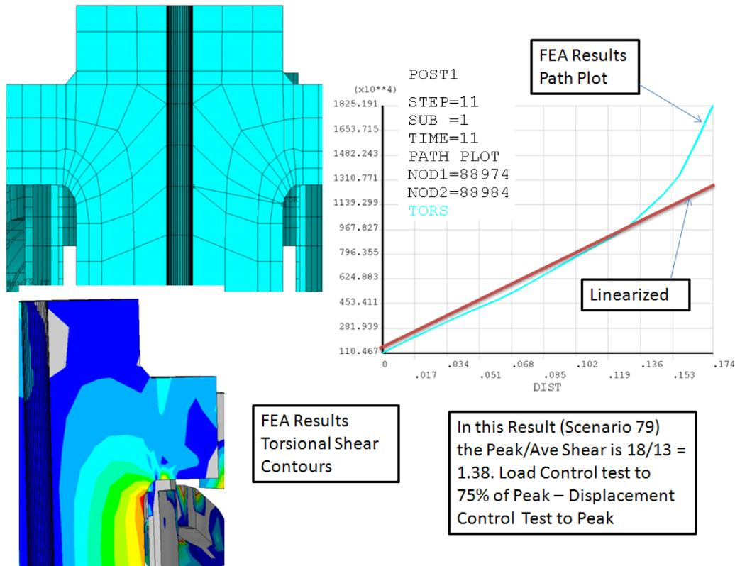
Figure 8a Linearized vs. Actual Shear Stress Distribution
