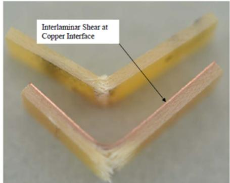
CTD-425 Specimen #14- Fatigue at 60% of Ultimate Stress (31 MPa, 26851 cycles)
