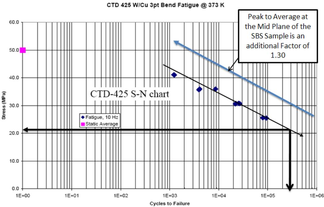
Figure 9d CTD Test Results With the Expected Higher Shear Capacity due to the Peaking of Stress in the Short Beam Shear Specimen
