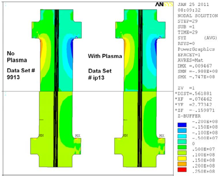
Figure 12 This shows one current set in which the plasma current effect on the torsional shear is difficult to discern.. From the influence coefficient calculations it is about a 1 MPa effect (see Figure 6). The magnitude is close to 20 MPa.
