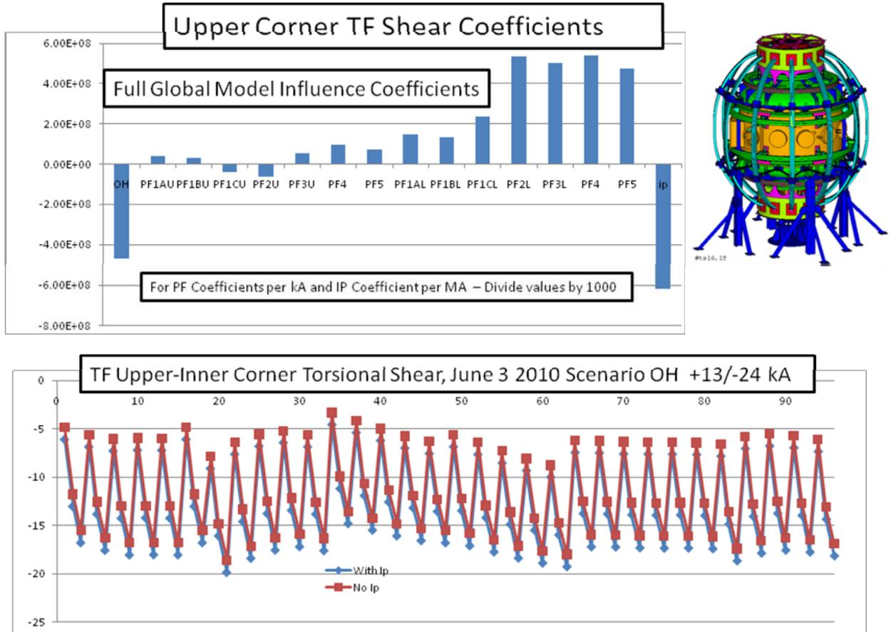
Figure 6 Torsional Shear Stresses from the influence coefficients multiplied by the Design Point Scenarios
