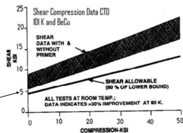
Figure 8b CDR Estimates of the NSTX Upgrade Shear Allowable
