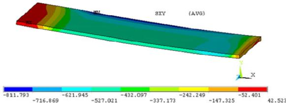
Shear Stress in the Copper and insulation interface is about 800 psi or 5 MPa
