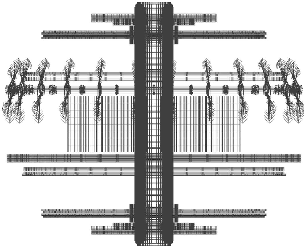
Figure 19 Forces on PF4u from a full TF current and 1 kA in PF4u. TF coils and forces have been removed to scale the much lower PF4 loads due to a kA terminal current.
