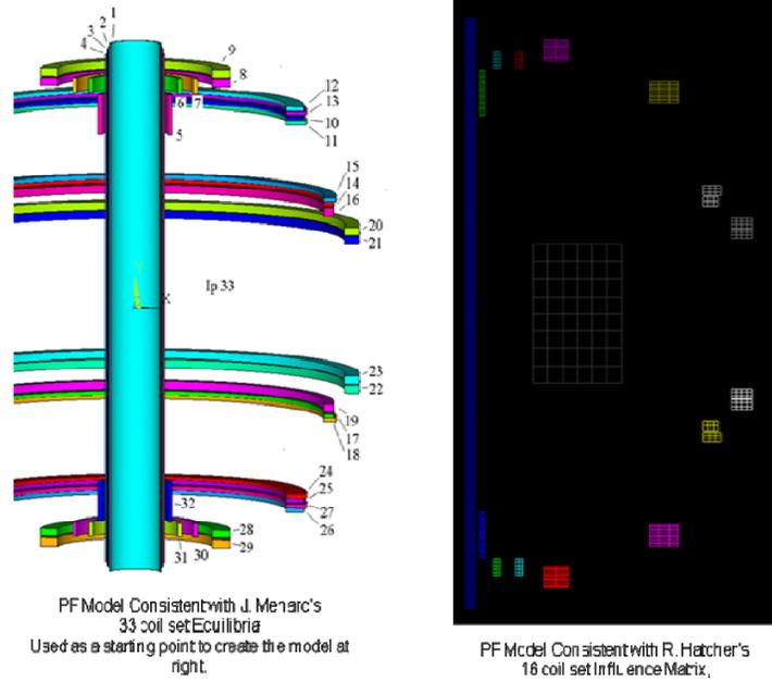
Figure 5 Coil Builds Used in the FEA analyses and the DCPS
