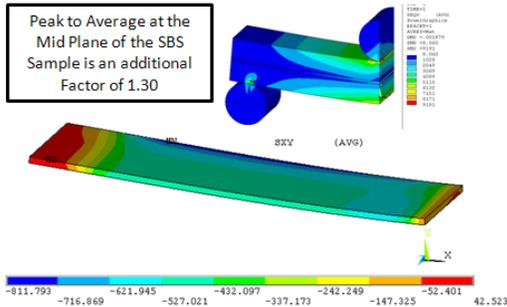
Figure 9c FDR Slide Showing Test Results, and Short Beam Shear Finite Element Model
