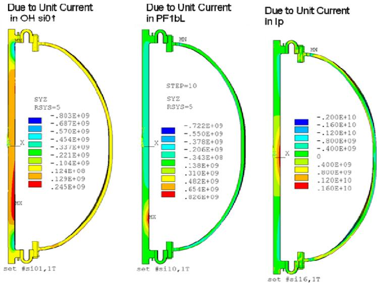
Figure 25 Single Coil Model Torsional Shear Contour Plots for 3 of the 16 Unit Loads
