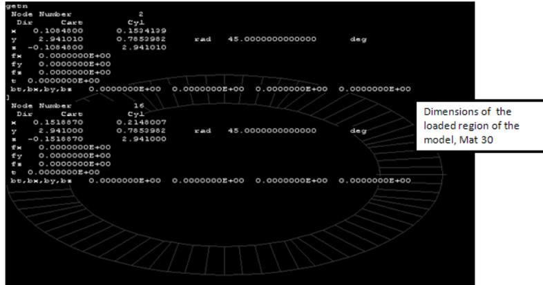
Applied Torque =  $72 * .1534139 + 72 * .2148 = 26.51 \text{ N-m}$
