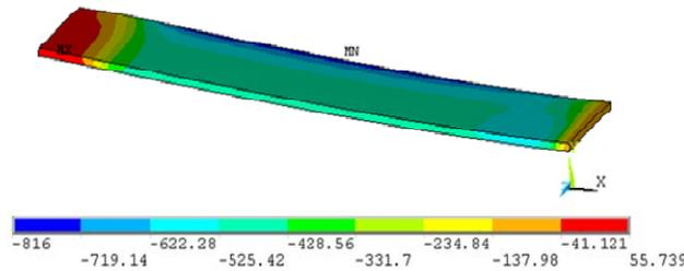
Shear Stress in the Copper and insulation interface is about 800 psi or 5 MPa
