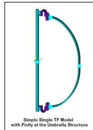
simpler model allows easier post processing, and with additions of stiffnesses replacing the imposed constraints, this scale of model could be useful. The results of this model are included mainly for illustration of the process (see Appendix B) and comparison with the global model results.
