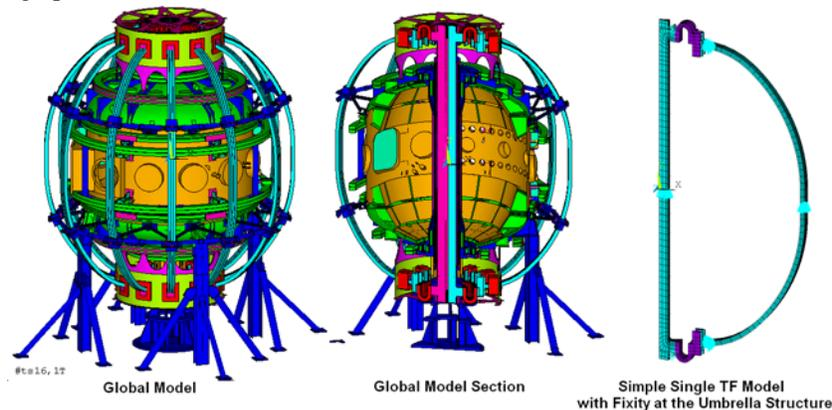
Figure 1 FEA Models Used for the Calculation of TF Inner Leg Shear Stress Influence Coefficients.
