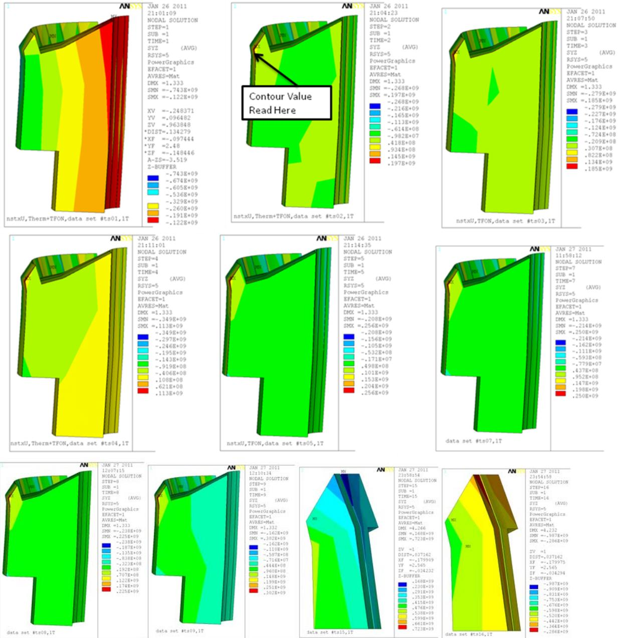
Figure 18 Selected Post Process Results from the upper Corner Shear Stress Influence Coefficients
