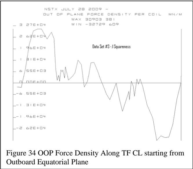
Figure 34 OOP Force Density Along TF CL starting from Outboard Equatorial Plane
