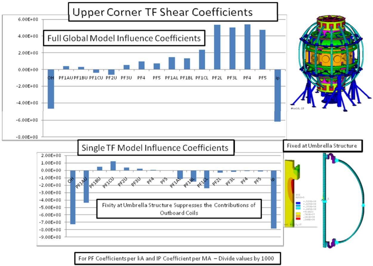
Figure 29 Comparison of Influence Coefficient Results for the Global and Single Coil Models
