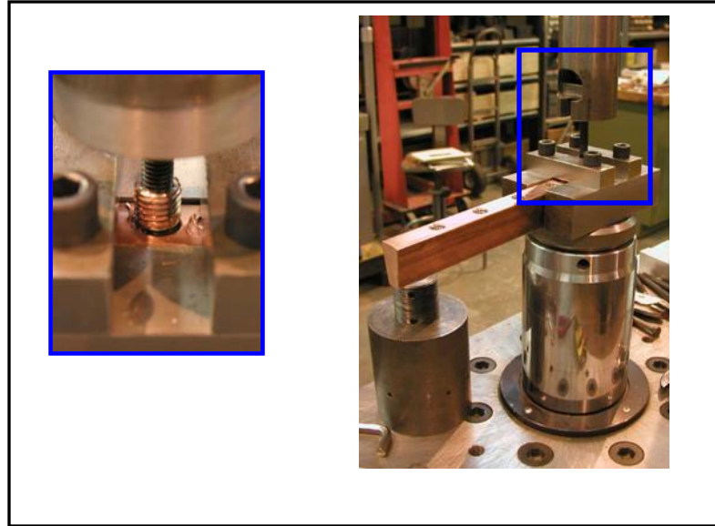
Figure 5 - 3/8-16 Tap-Lok Insert/ C10700 Copper Thread Pull-Out Test
