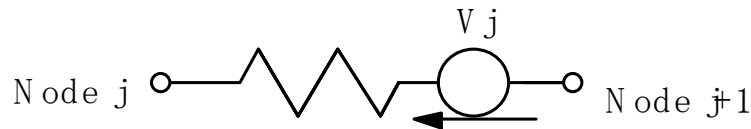
Figure 20: Thevenin Equivalent of the Fig.21 Circuit, Using A Voltage Source
