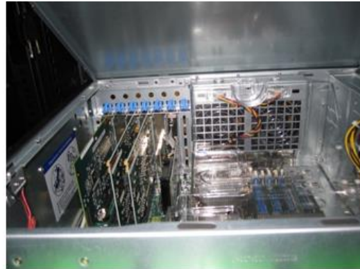
Internal View of DCPS Computer with I/O cards installed
