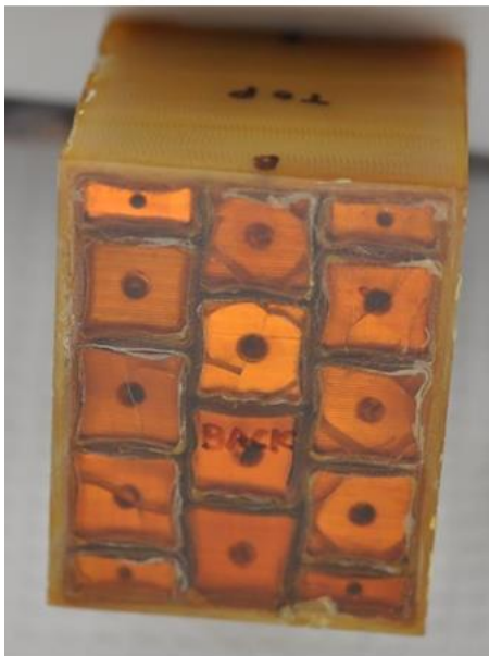
Figure 17.2-3 Array Test Sample from [23] (The sample at left was shortened in the actual tests) The CTD aligned conductor tests show a significant accommodation of tensile strains. The tests are displacement or strain controlled, performed at 110 C at a strain amplitude of 0.4 \times 10^{-3} and a rate of \sim 10 hz. A full discussion of these tests and their application to the OH can be found in [21] While the electrical
