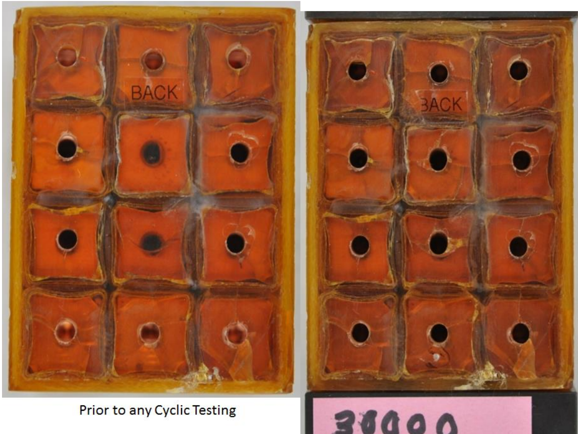
Figure 4.0-15 CTD Tensile Strain Controlled Test, Aligned Sample
