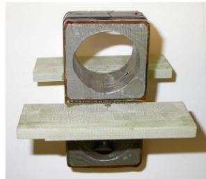
Figure 6.4-2 MIT tests of Insulation with Interleaved Kapton/glass
