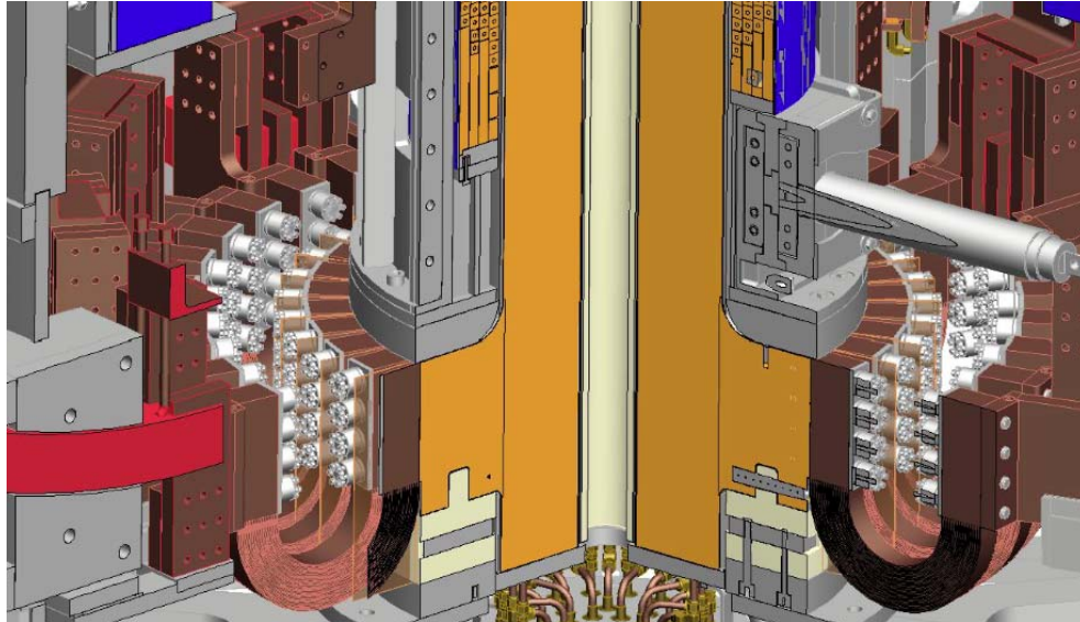
Figure 13.0-2 Lower OH Support Area – There Aren't Cracks or Open Areas for powdered Aquapour to Escape
