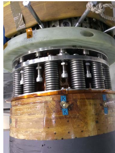
Figure 15.0-1 Torsional Creep Tests Performed at MAST and the NSTX Preload Mechanism
