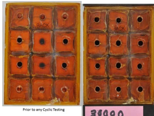
Fig. 14.0-7 CTD Tensile Strain Controlled Test, Aligned Sample
