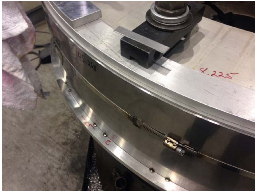
Figure 6.3-2 Photo of the Outer Shell Welding
