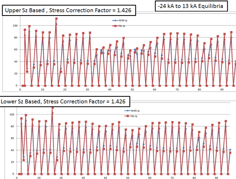
Figure 3.0-2 Hoop Stresses for the Design Equilibria Upper and Lower Coil Regions
