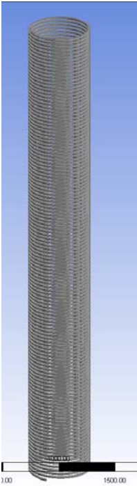
Fig. 2 OH winding showing one of the eight cooling paths
